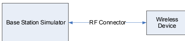
Figure 9-1 Power Measurement Setup
