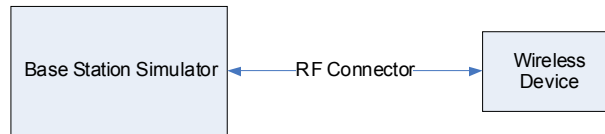
Figure 9-2 Power Measurement Setup
