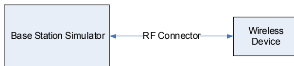
Figure 8-1 Power Measurement Setup
