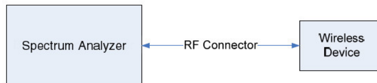
Figure 7-1. Test Instrument & Measurement Setup
