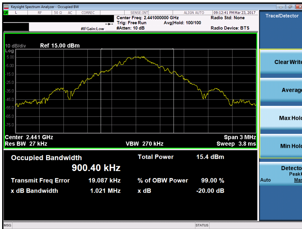
Plot 7-2. 20dB Bandwidth Plot (Bluetooth, 1Mbps – Ch. 39)
