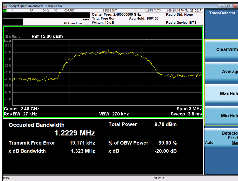
Plot 7-9. 20dB Bandwidth Plot (Bluetooth, 3Mbps – Ch. 78)
