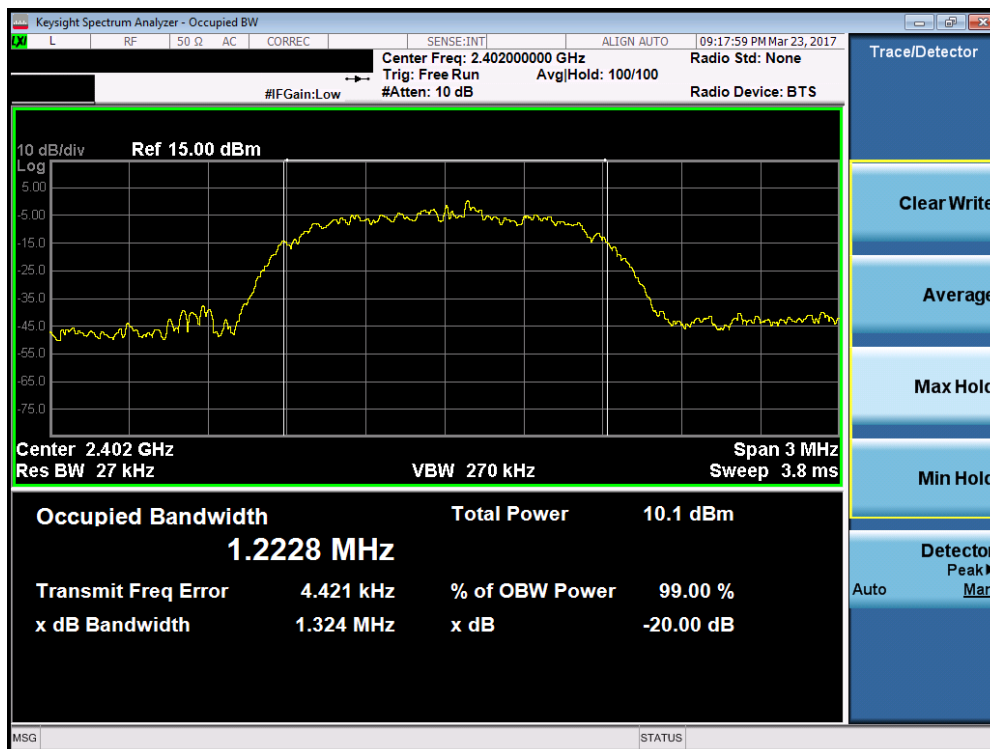
Plot 7-7. 20dB Bandwidth Plot (Bluetooth, 3Mbps – Ch. 0)
