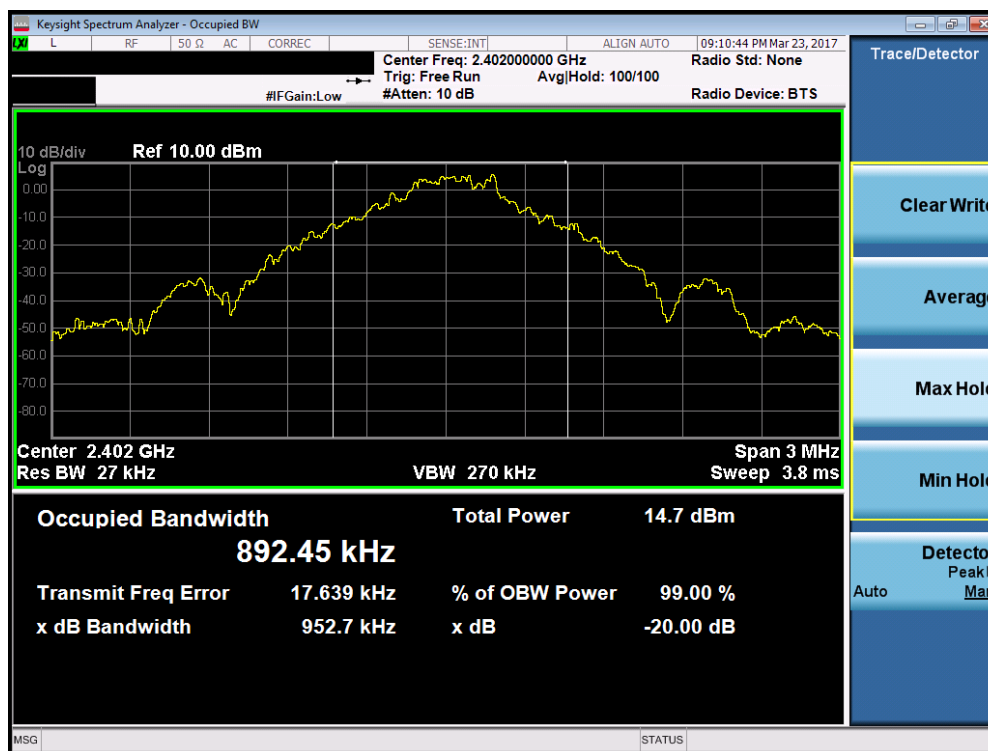
Plot 7-1. 20dB Bandwidth Plot (Bluetooth, 1Mbps – Ch. 0)
