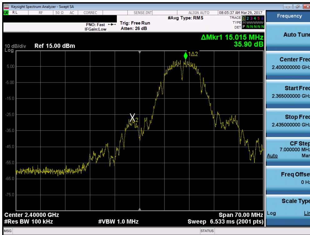
Plot 7-19. Band Edge Plot (802.11b – Ch. 1)
