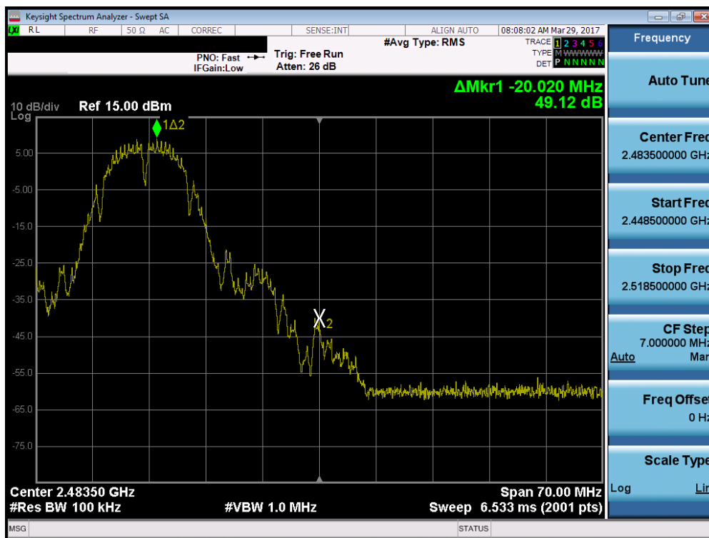
Plot 7-20. Band Edge Plot (802.11b – Ch. 11)
