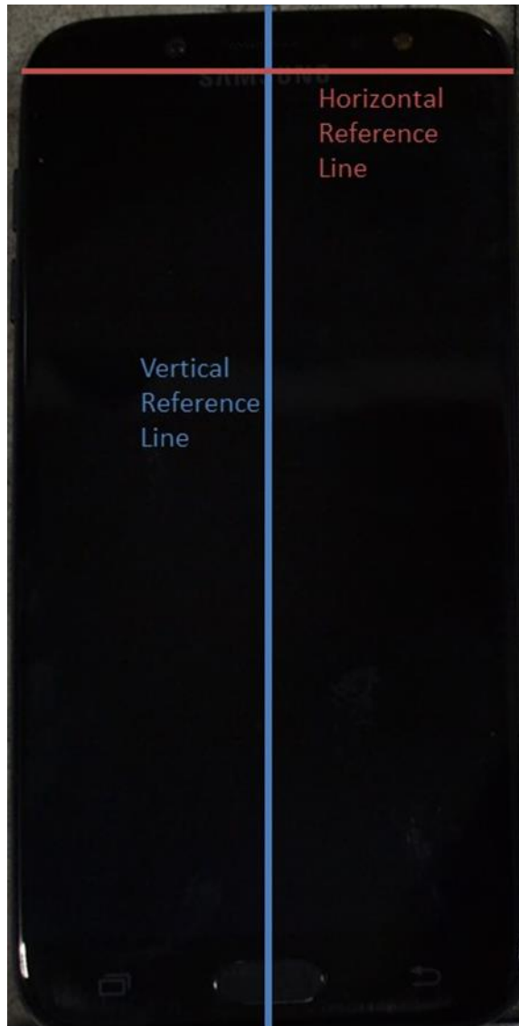
SAR Test Setup Photo 21- Horizontal and Vertical Reference Lines
