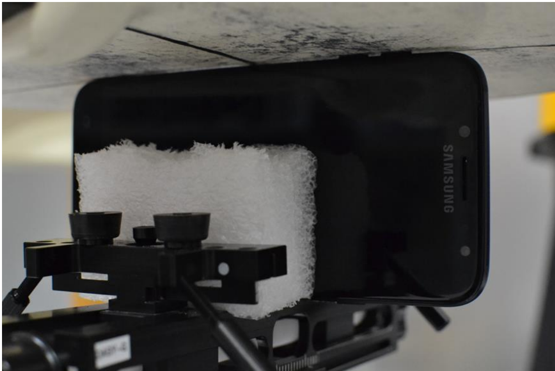
SAR Test Setup Photo 20- Left Edge at 0.0 cm (Phablet)
