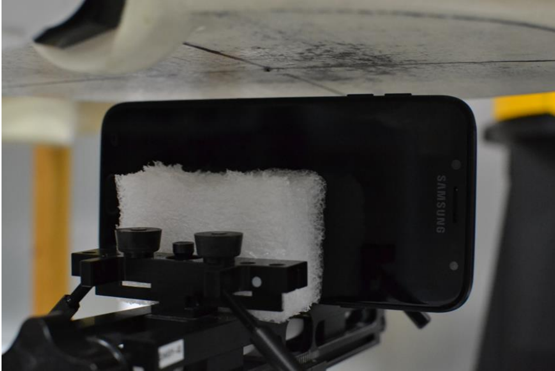
SAR Test Setup Photo 19- Left Edge at 1.0 cm (Hotspot)
