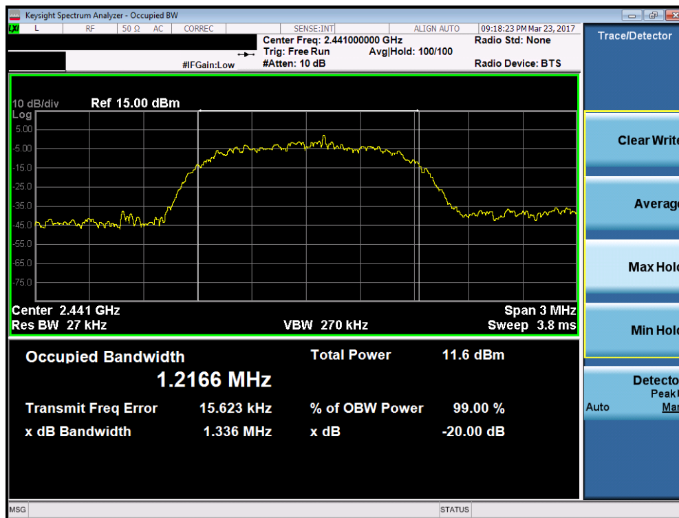
Plot 7-8. 20dB Bandwidth Plot (Bluetooth, 3Mbps – Ch. 39)
