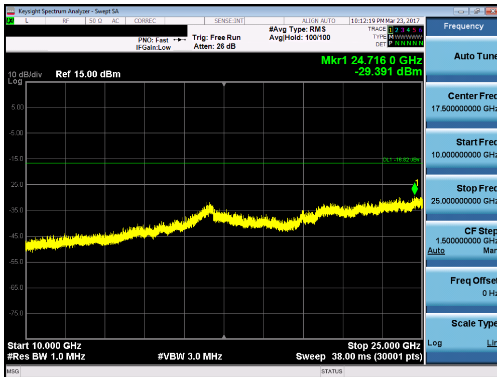
Plot 7-37. Conducted Spurious Plot (Bluetooth, 1Mbps – Ch. 0)
