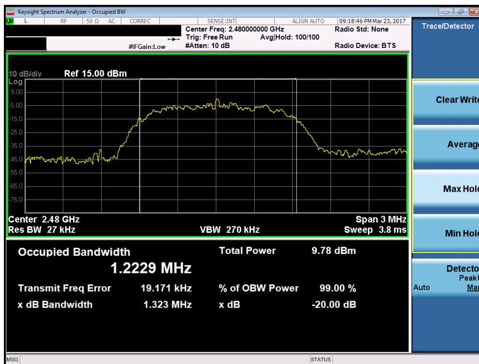
Plot 7-9. 20dB Bandwidth Plot (Bluetooth, 3Mbps – Ch. 78)
