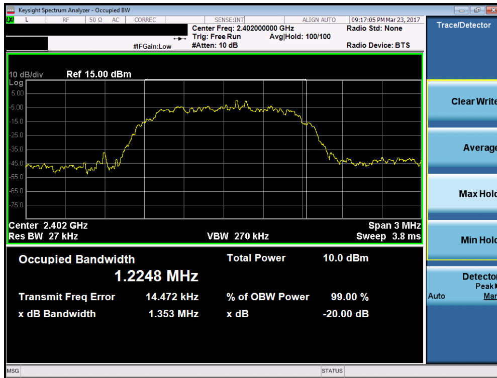
Plot 7-4. 20dB Bandwidth Plot (Bluetooth, 2Mbps – Ch. 0)
