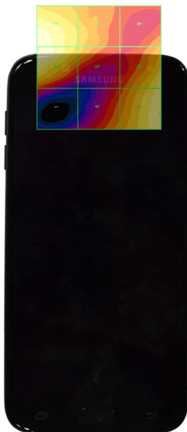
Figure 18-4 E-Field WD Scan overlay
