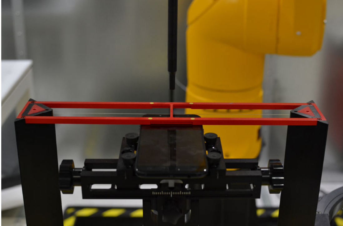
Figure 18-1 Ear Reference Point HAC Phantom Alignment
