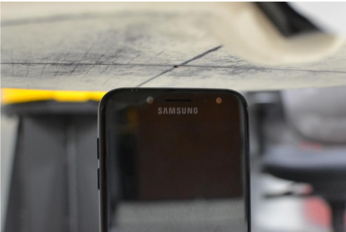
SAR Test Setup Photo 12- Top Edge at 1.0 cm (Hotspot)
