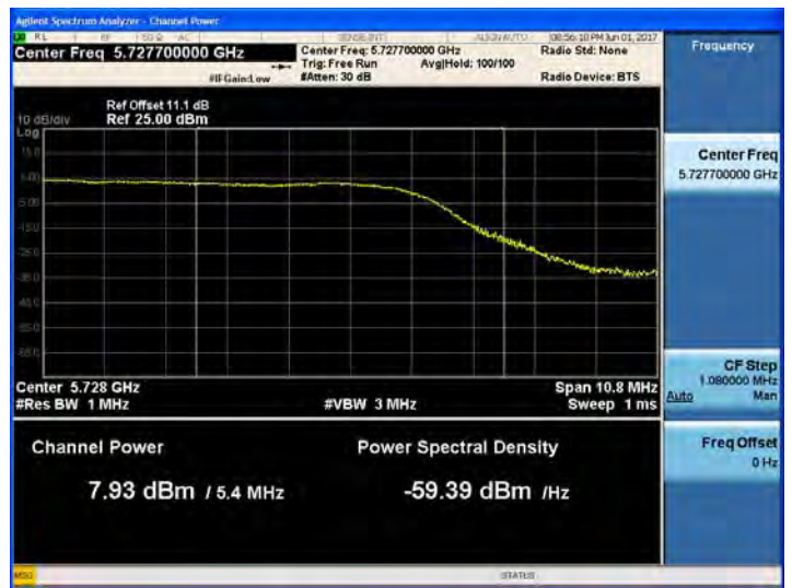
802.11ac_VHT20 UNII 3 Band Average Power CH.144
