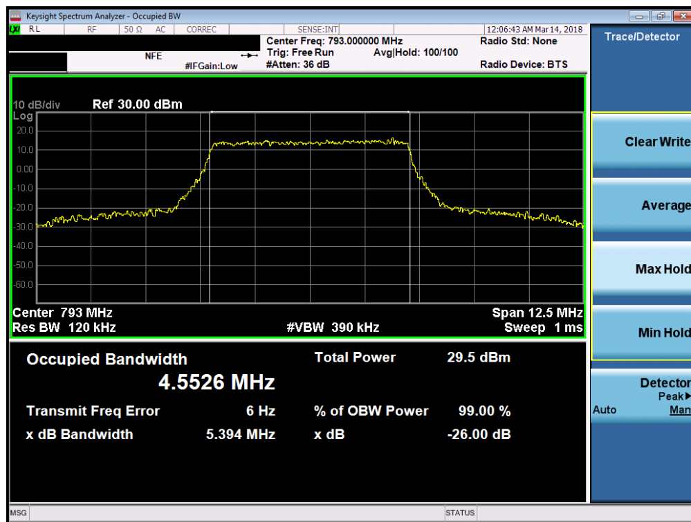
Plot 7-1. Occupied Bandwidth Plot (LTE B14 - 5MHz QPSK – RB Size 25)
