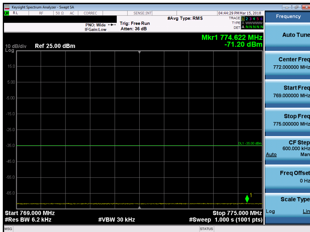
Plot 7-19. Lower Emission Mask Band Edge Plot (LTE B14 - 10MHz QPSK – RB Size 50)
