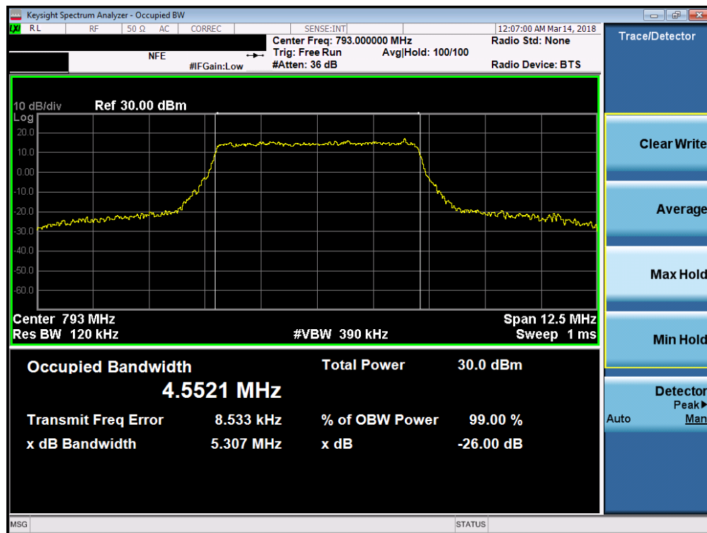
Plot 7-2. Occupied Bandwidth Plot (LTE B14 - 5MHz 16-QAM – RB Size 25)
