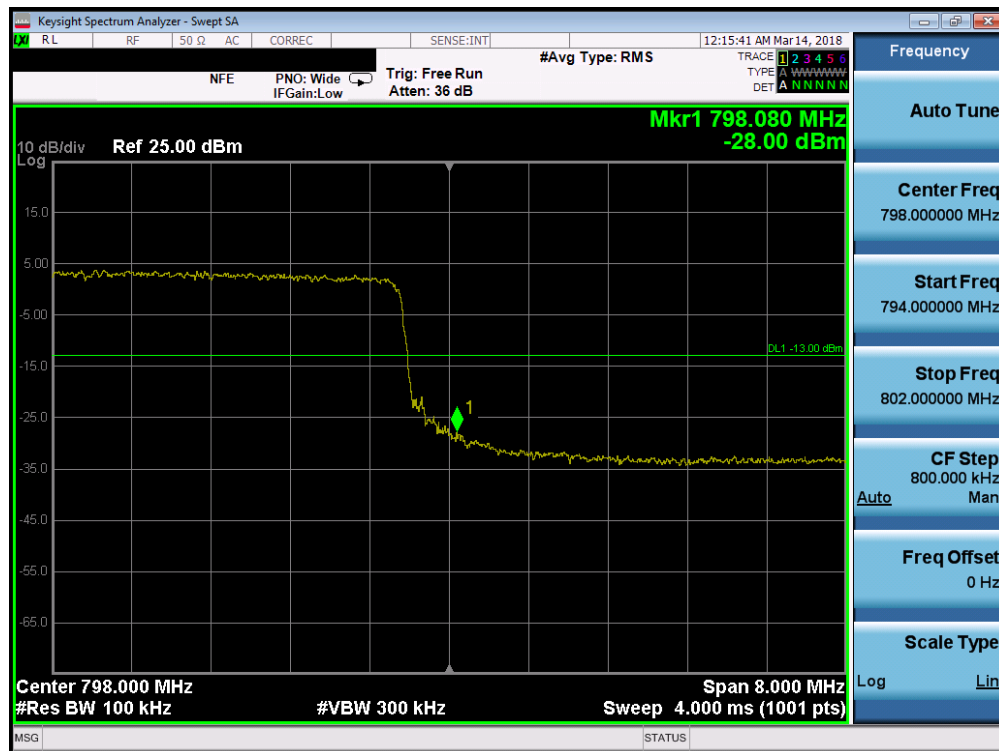
Plot 7-20. Upper Band Edge Plot (LTE B14 - 10MHz QPSK - RB Size 50)
