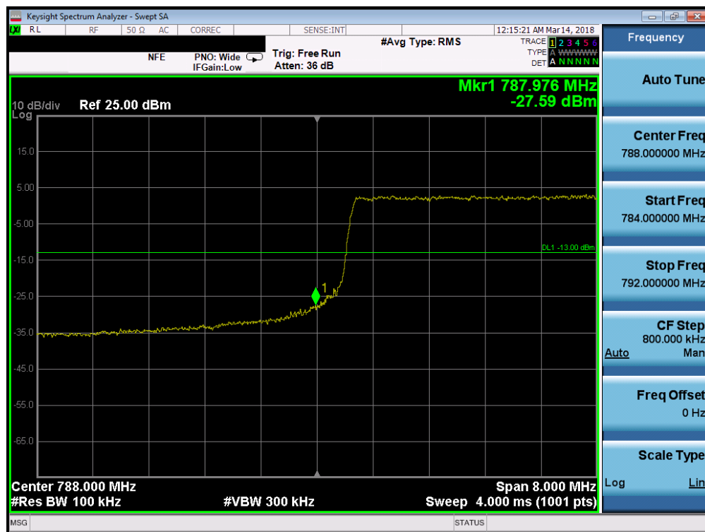
Plot 7-18. Lower Band Edge Plot (LTE B14 - 10MHz QPSK – RB Size 50)
