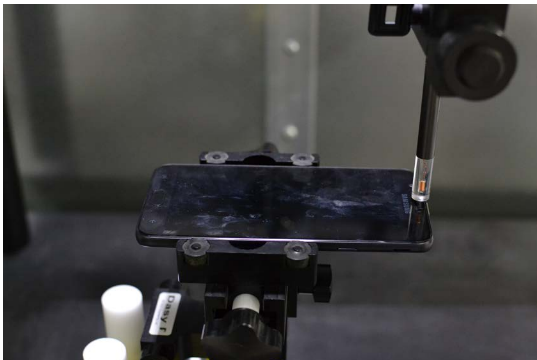
Figure 16-1 Test Setup for Wireless Device
