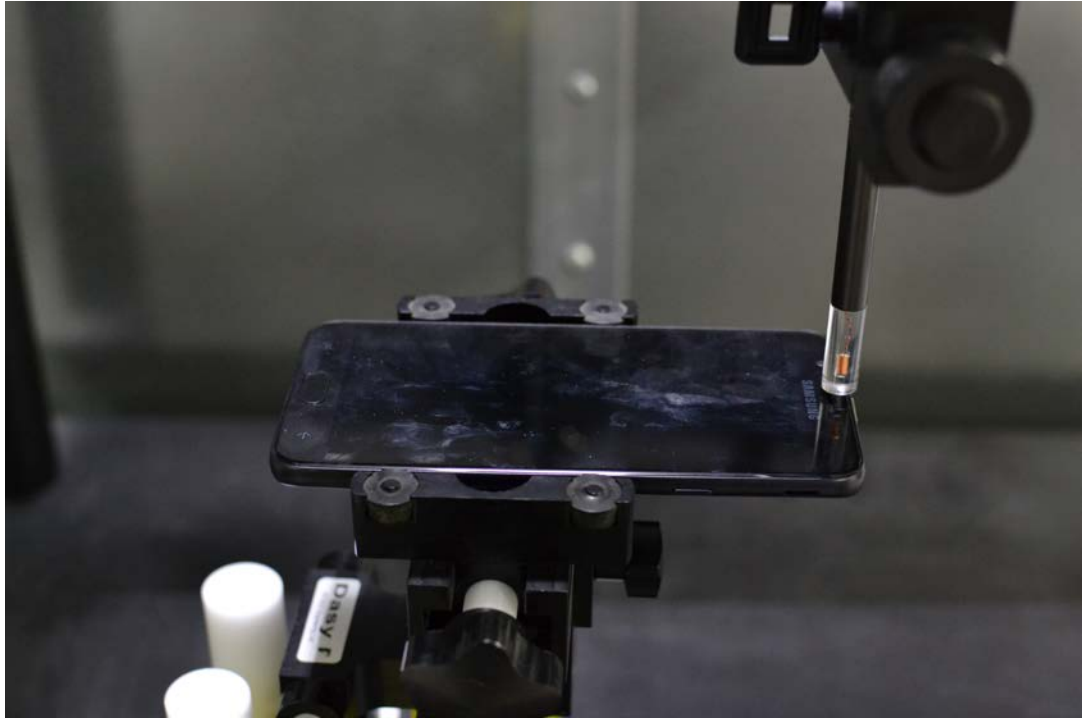
Figure 16-1 Test Setup for Wireless Device
