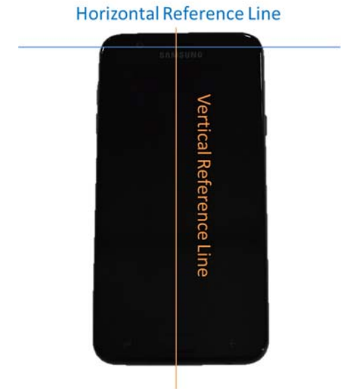
SAR Test Setup Photo 21 Reference Lines
