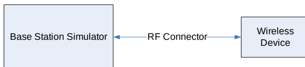
Figure 9-1 Power Measurement Setup
