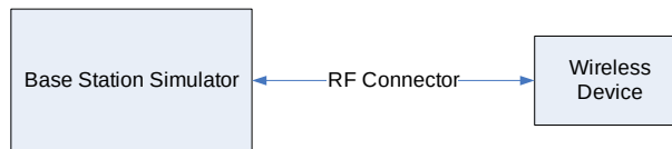
Figure 9-2 Power Measurement Setup
