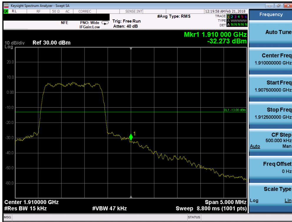
Plot 7-85. Band Edge Plot (PCS CDMA Mode - High Channel)
