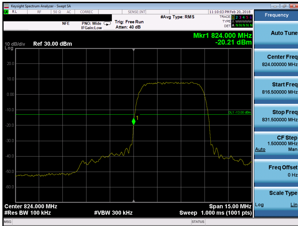
Plot 7-87. Band Edge Plot (Cellular WCDMA Mode - Low Channel)
