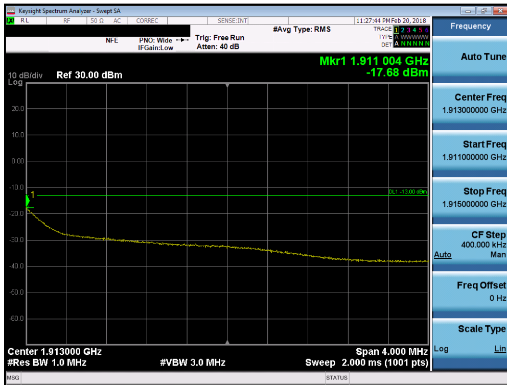
Plot 7-96. 4MHz Span Plot (PCS WCDMA Mode - High Channel)
