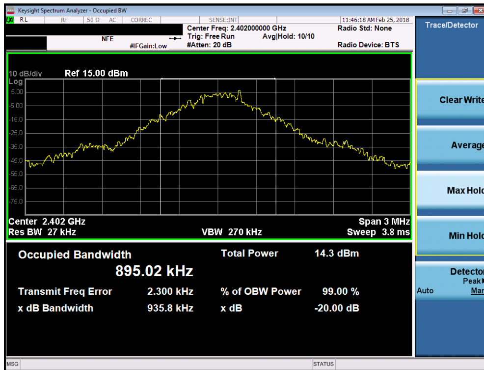
Plot 7-1. 20dB Bandwidth Plot (Bluetooth, 1Mbps – Ch. 0)
