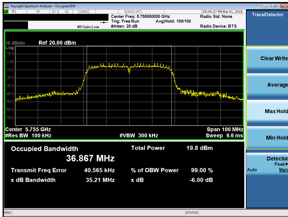
Plot 7-37. 6dB Bandwidth Plot (40MHz BW 802.11n (UNII Band 3) – Ch. 151)
