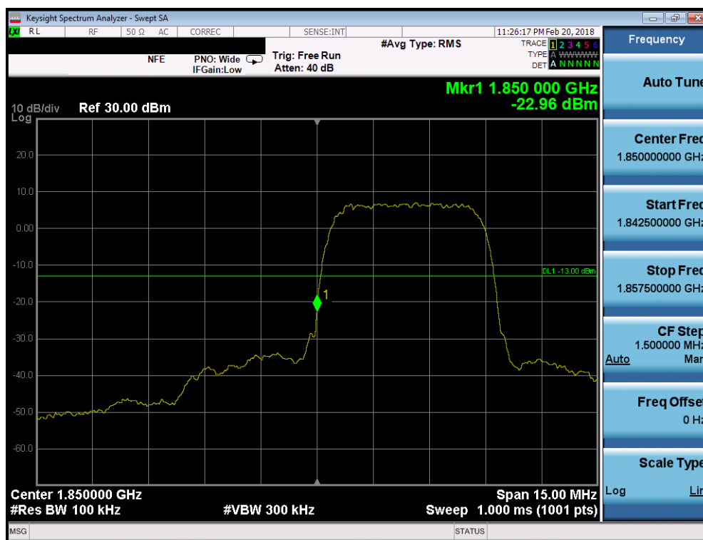
Plot 7-79. Band Edge Plot (PCS WCDMA Mode - Low Channel)
