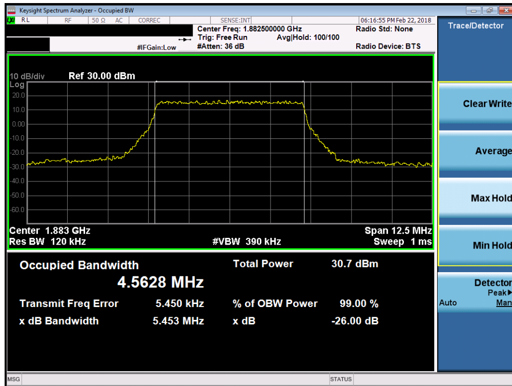
Plot 7-33. Occupied Bandwidth Plot (Band 25/2 - 5.0MHz QPSK - Full RB Configuration)
