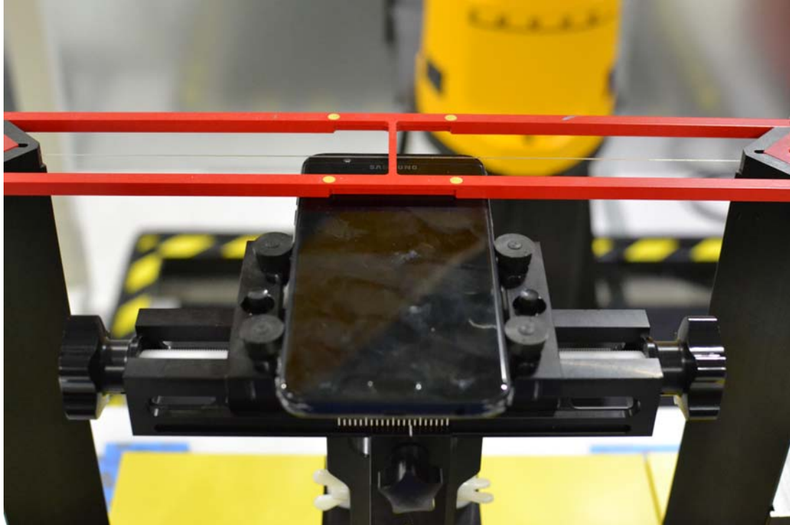
Figure 17-1 Ear Reference Point HAC Phantom Alignment
