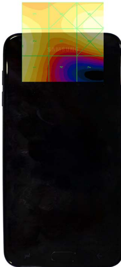
Figure 17-4 E-Field WD Scan overlay
