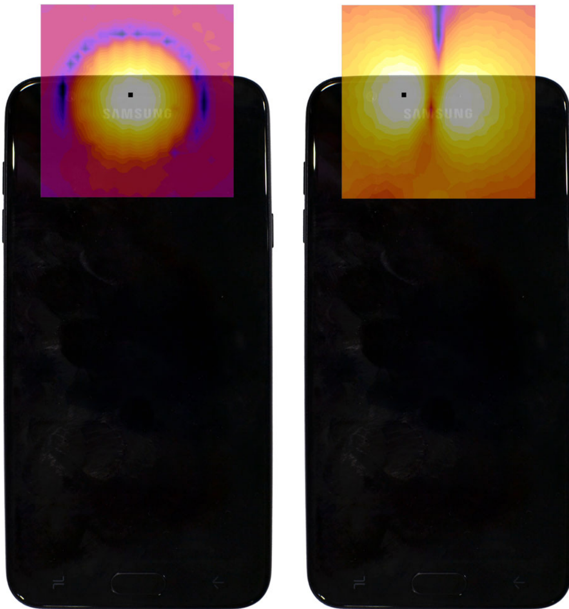
Figure 15-3 T-Coil Scan Overlay Magnetic Field Distributions
