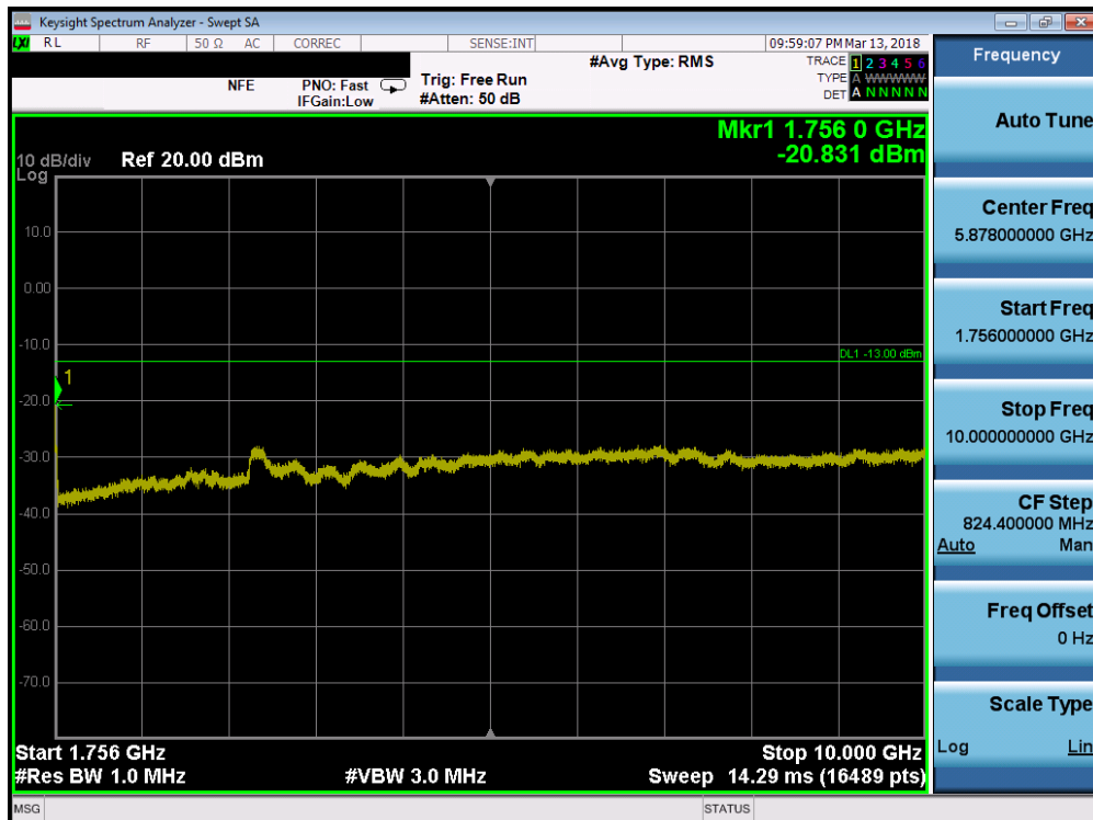
Plot 7-91. Conducted Spurious Plot (Band 66/4 - 20.0MHz QPSK - RB Size 1, RB Offset 0 - High Channel)
