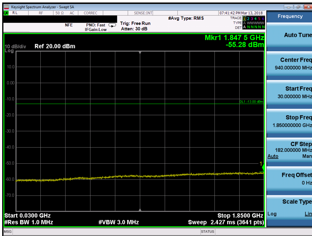
Plot 7-96. Conducted Spurious Plot (Band 2 - 5.0MHz QPSK - RB Size 1, RB Offset 0 - Mid Channel)
