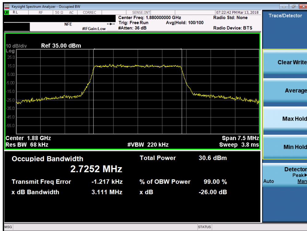
Plot 7-39. Occupied Bandwidth Plot (Band 2 - 3.0MHz QPSK - Full RB Configuration)
