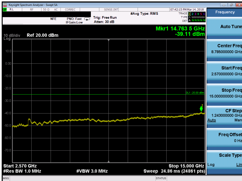
Plot 7-103. Conducted Spurious Plot (Band 7 - 10.0MHz QPSK - RB Size 1, RB Offset 0 - Low Channel)
