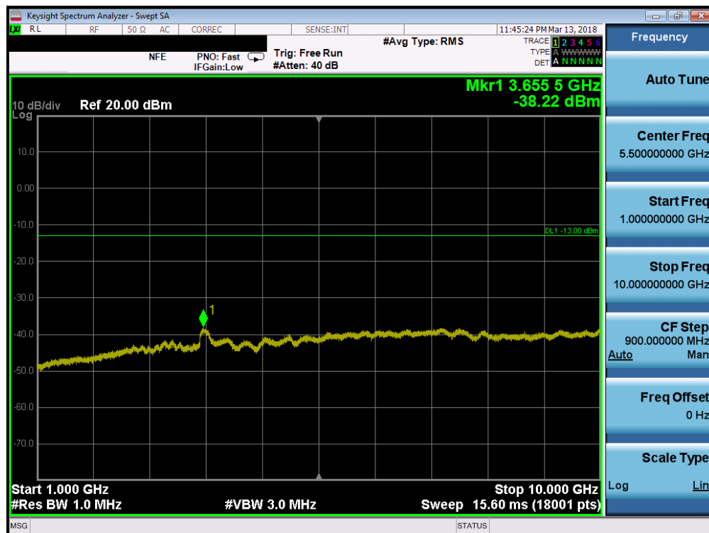
Plot 7-71. Conducted Spurious Plot (Band 12 - 3.0MHz QPSK - RB Size 1, RB Offset 0 - Mid Channel)
