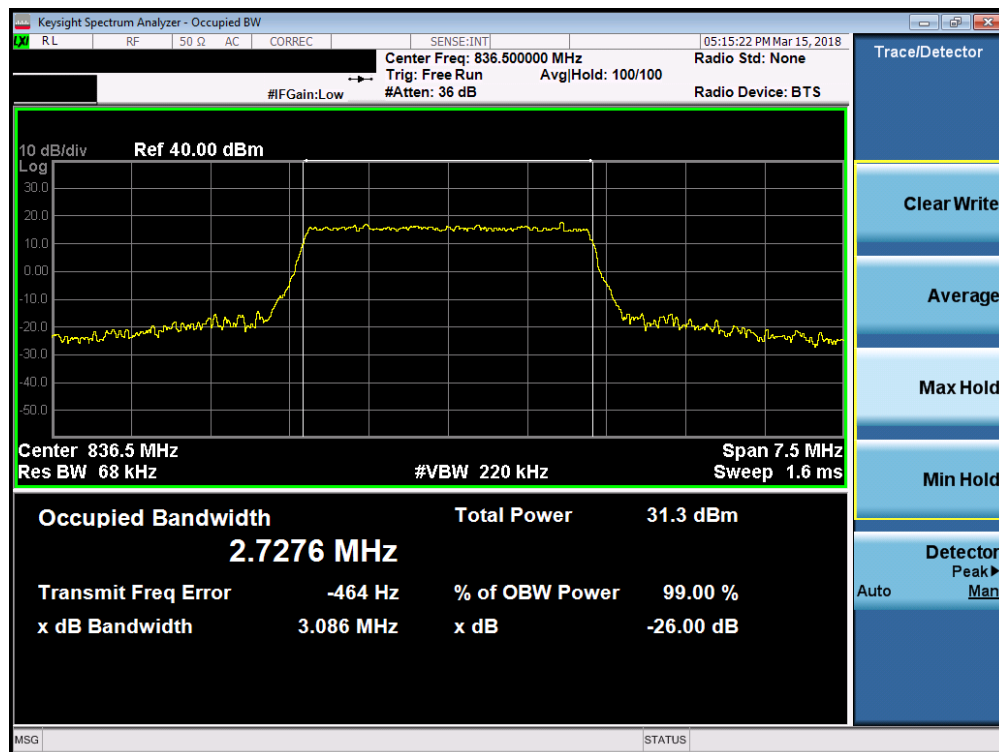
Plot 7-20. Occupied Bandwidth Plot (Band 5 - 3.0MHz 16-QAM - Full RB Configuration)
