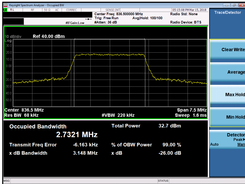
Plot 7-19. Occupied Bandwidth Plot (Band 5 - 3.0MHz QPSK - Full RB Configuration)
