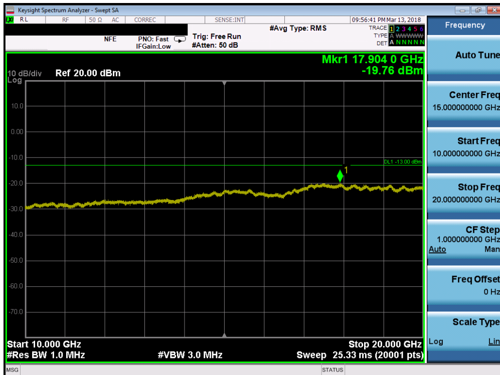
Plot 7-89. Conducted Spurious Plot (Band 66/4 - 20.0MHz QPSK - RB Size 1, RB Offset 0 - Mid Channel)
