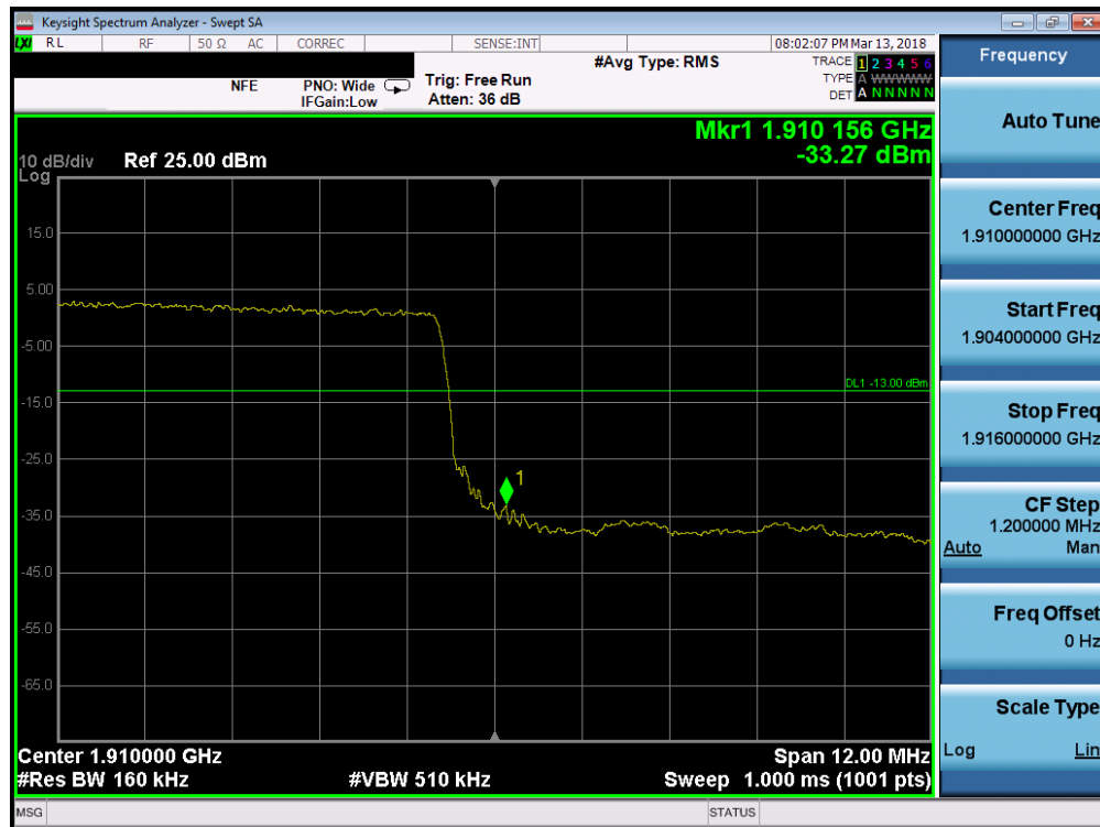
Plot 7-191. Upper Band Edge Plot (Band 2 - 15.0MHz QPSK - Full RB Configuration)
