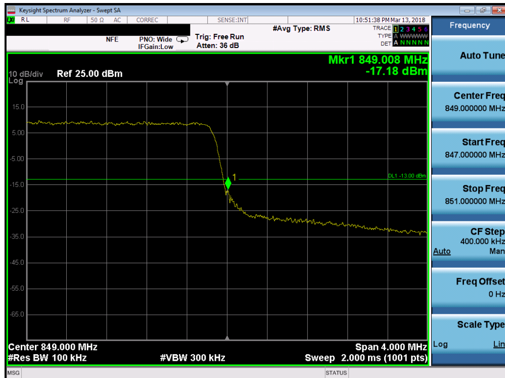
Plot 7-132. Upper Band Edge Plot (Band 5 - 3.0MHz QPSK - Full RB Configuration)
