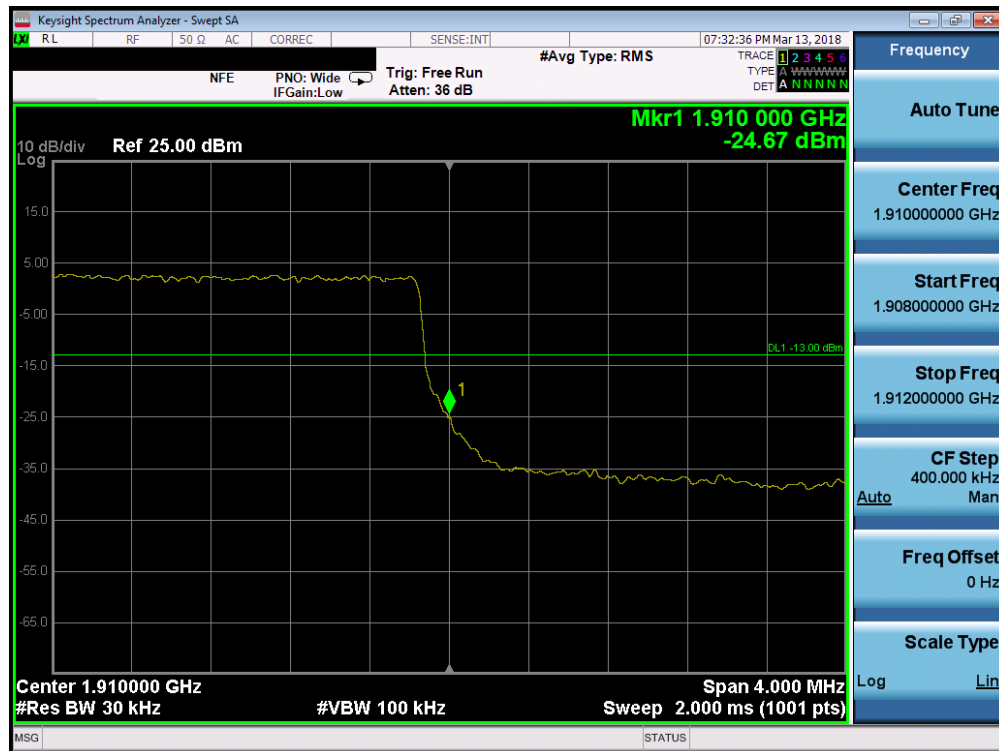
Plot 7-179. Upper Band Edge Plot (Band 2 - 3.0MHz QPSK - Full RB Configuration)
