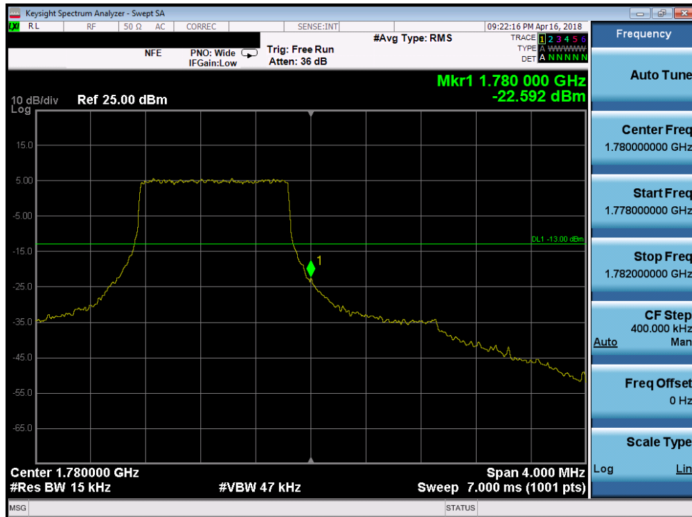
Plot 7-141. Upper Band Edge Plot (Band 66 - 1.4MHz QPSK - Full RB Configuration)
