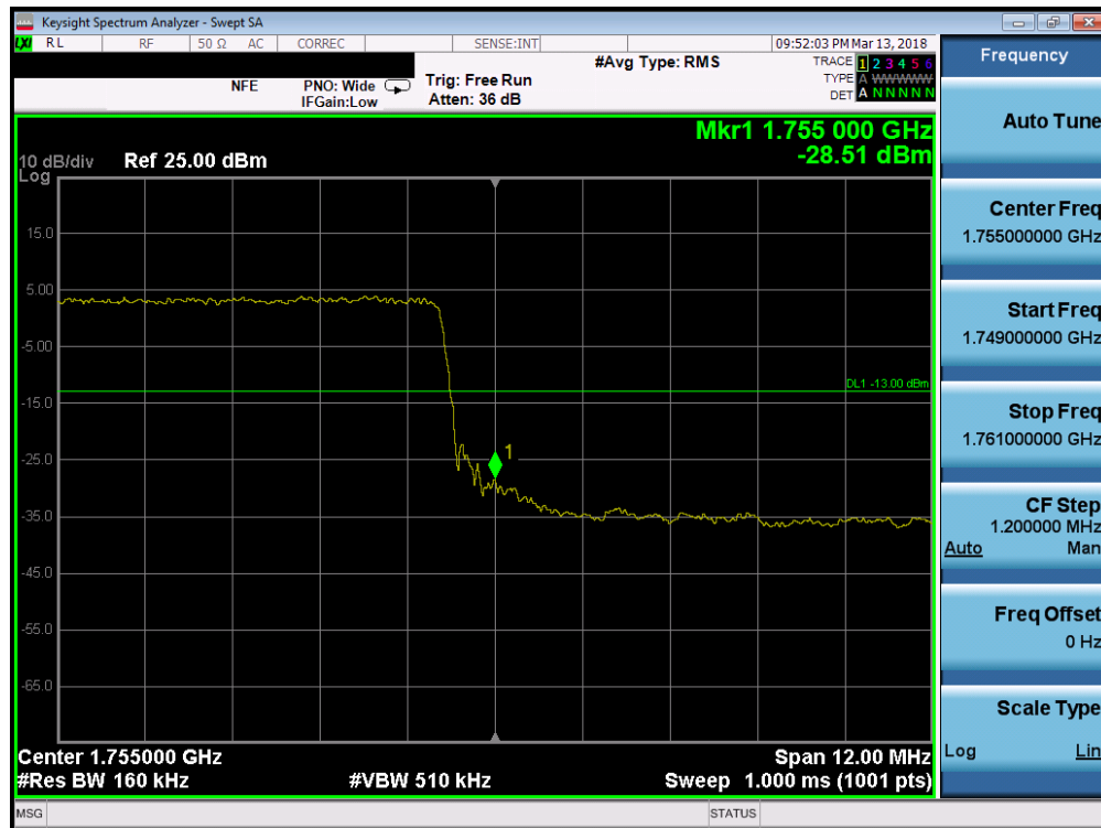
Plot 7-163. Upper Band Edge Plot (Band 4 - 15.0MHz QPSK - Full RB Configuration)
