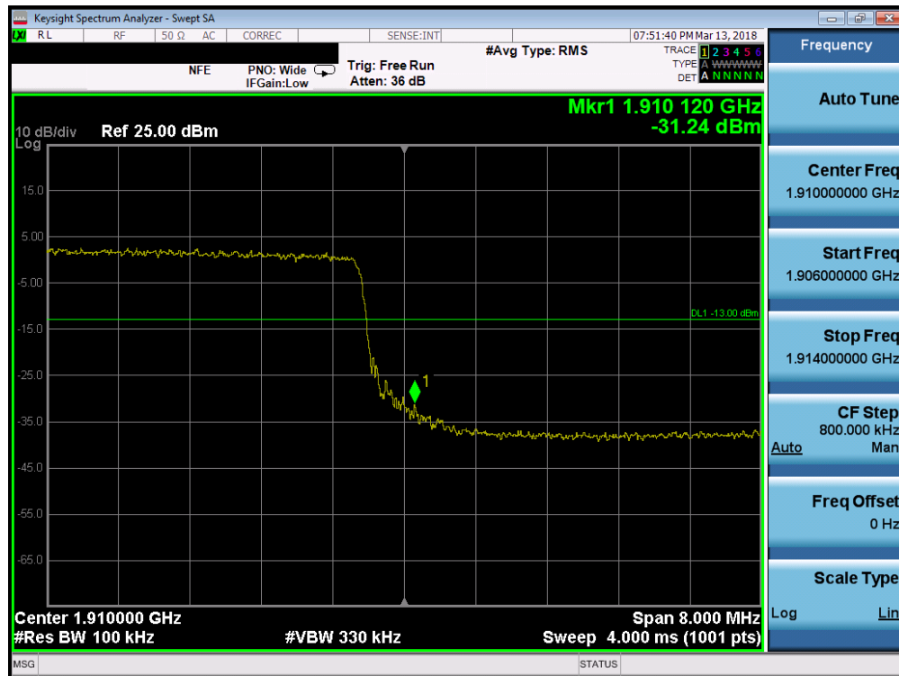
Plot 7-187. Upper Band Edge Plot (Band 2 - 10.0MHz QPSK - Full RB Configuration)
