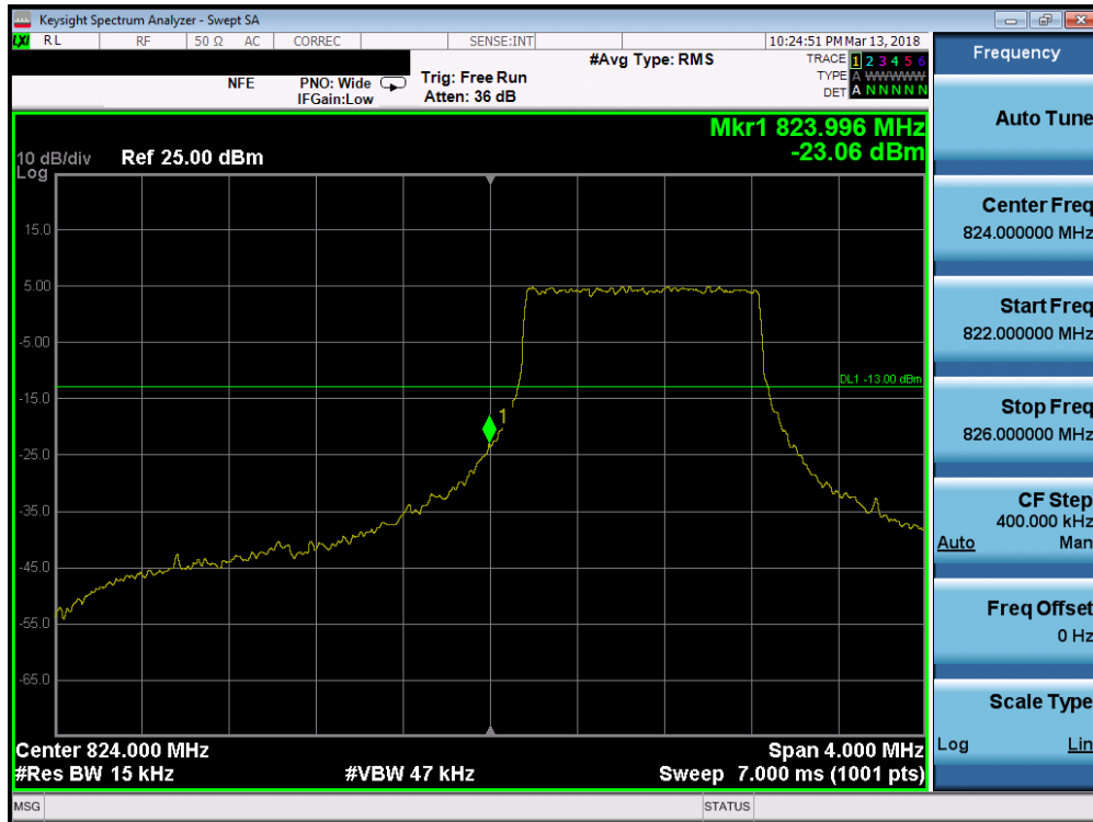
Plot 7-127. Lower Band Edge Plot (Band 5 - 1.4MHz QPSK - Full RB Configuration)
