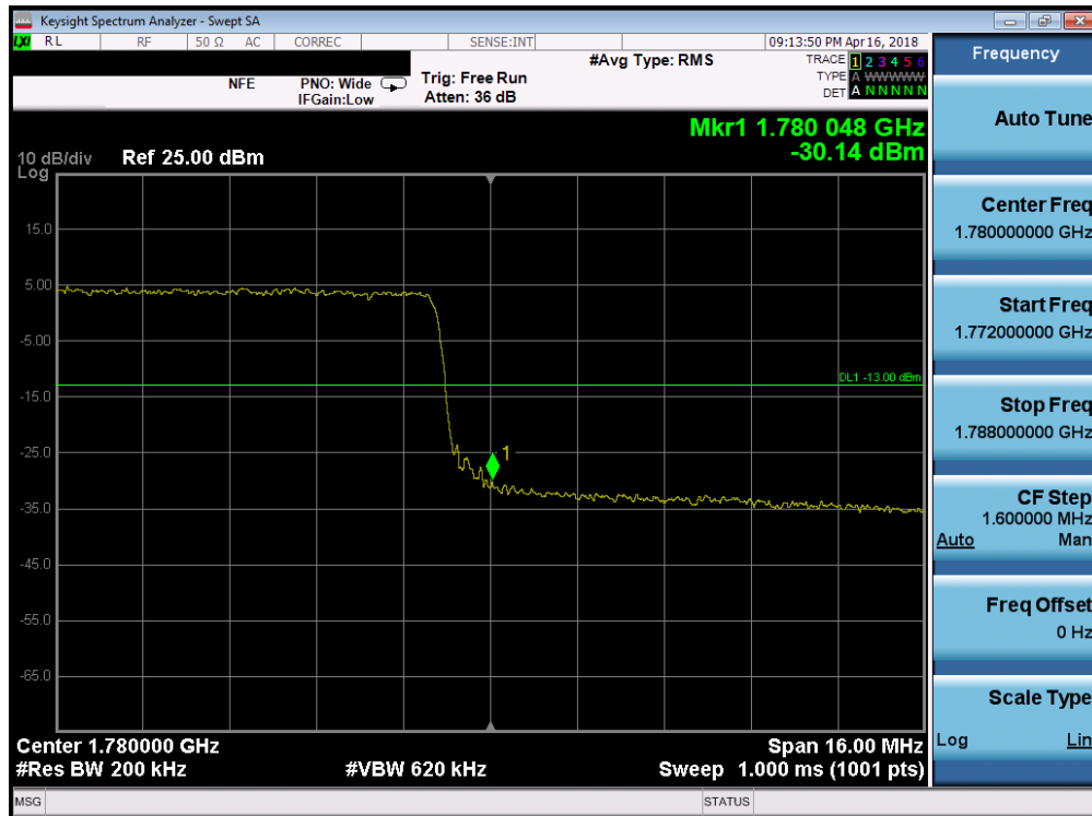
Plot 7-171. Upper Band Edge Plot (Band 66 - 20.0MHz QPSK - Full RB Configuration)
