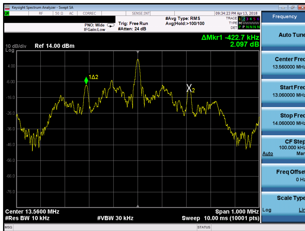
Figure 7-2. 20dB Bandwidth Plot
