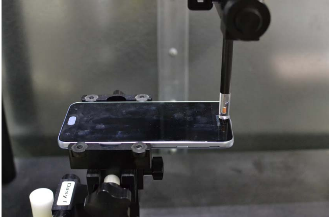
Figure 16-1 Test Setup for Wireless Device
