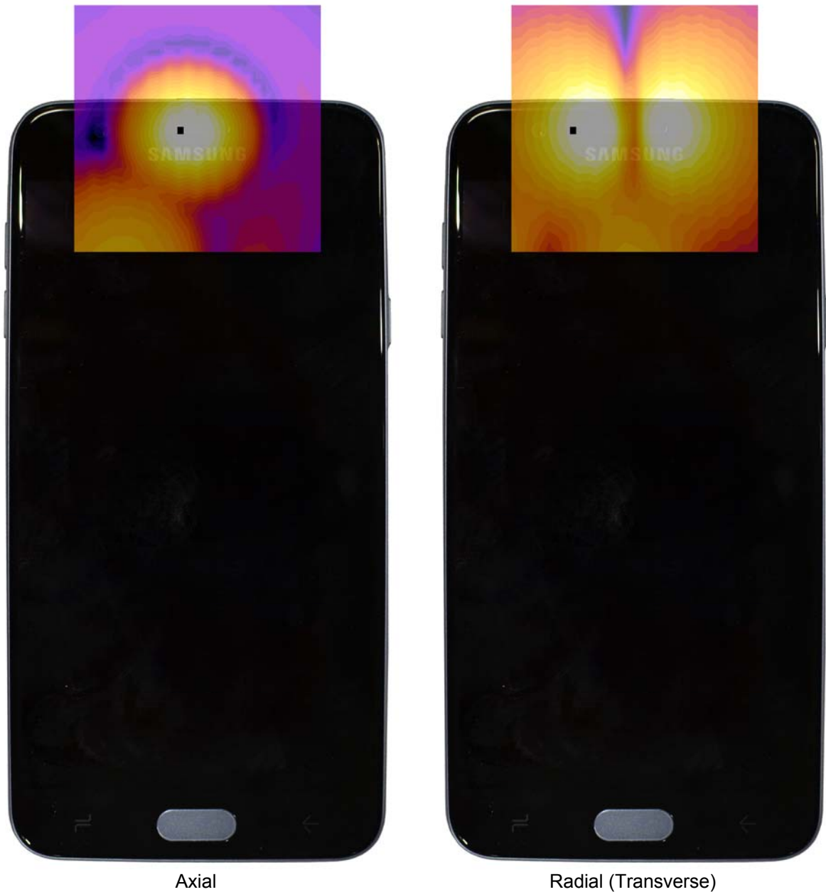
Figure 16-3 T-Coil Scan Overlay Magnetic Field Distributions
