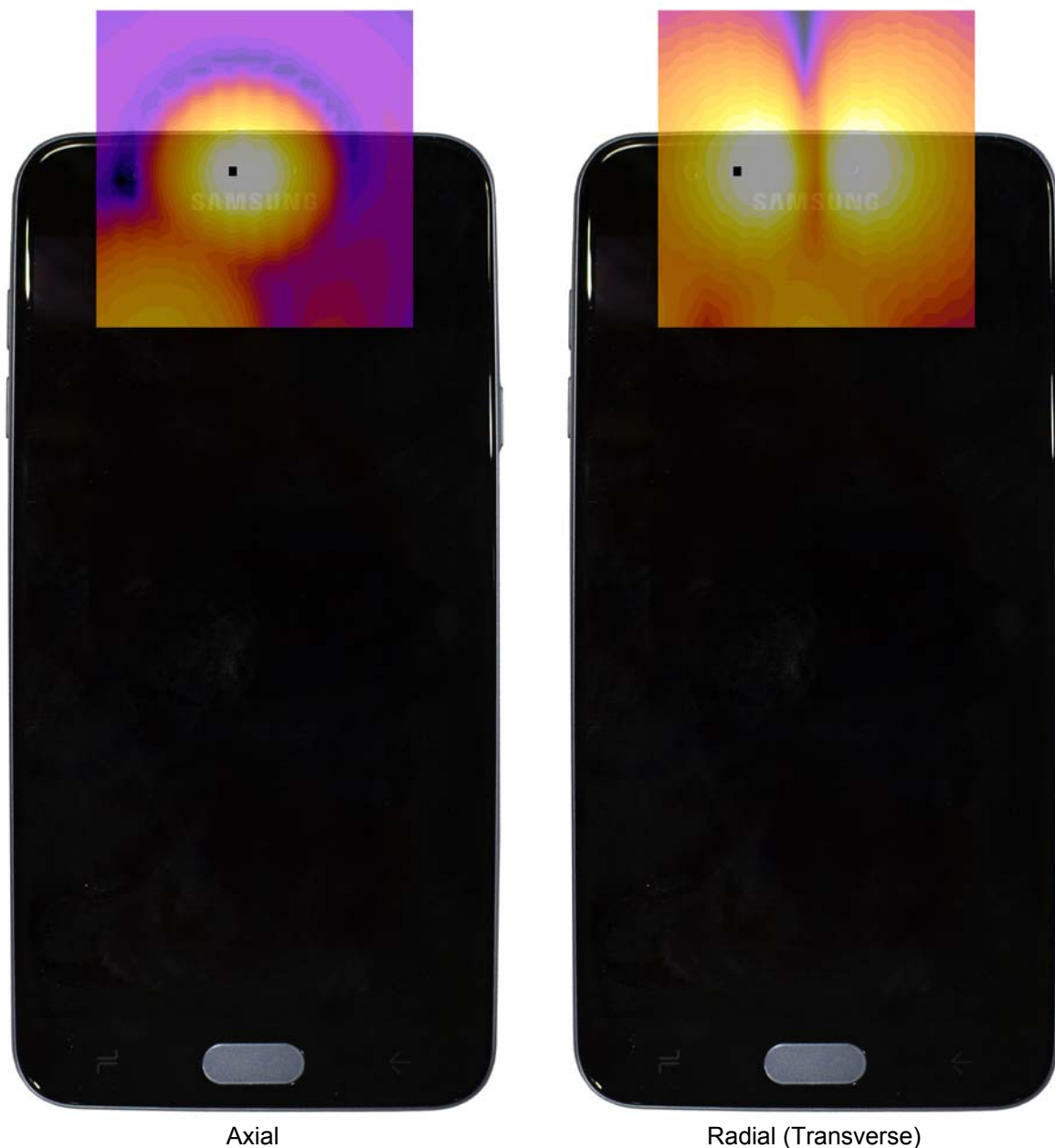
Figure 16-3 T-Coil Scan Overlay Magnetic Field Distributions
