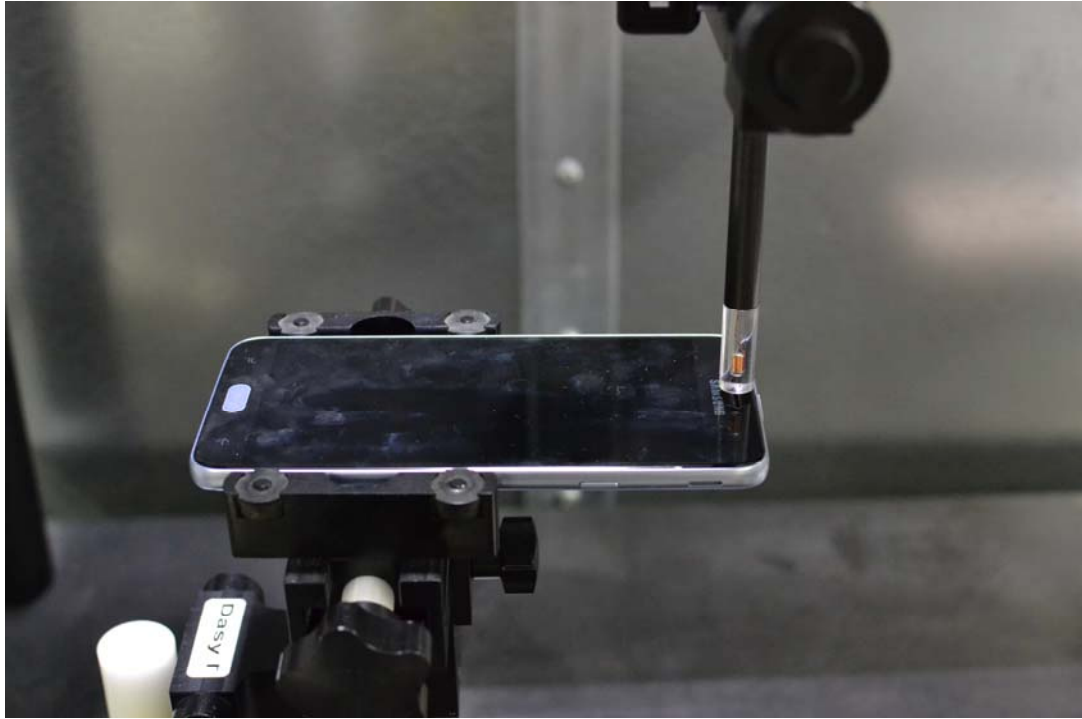
Figure 16-1 Test Setup for Wireless Device
