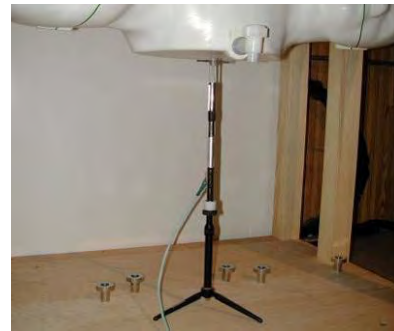
Figure 10-2 System Verification Setup Photo
