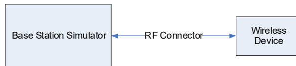
Figure 9-1 Power Measurement Setup
