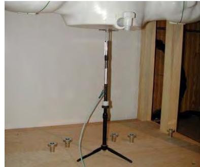
Figure 10-2 System Verification Setup Photo
