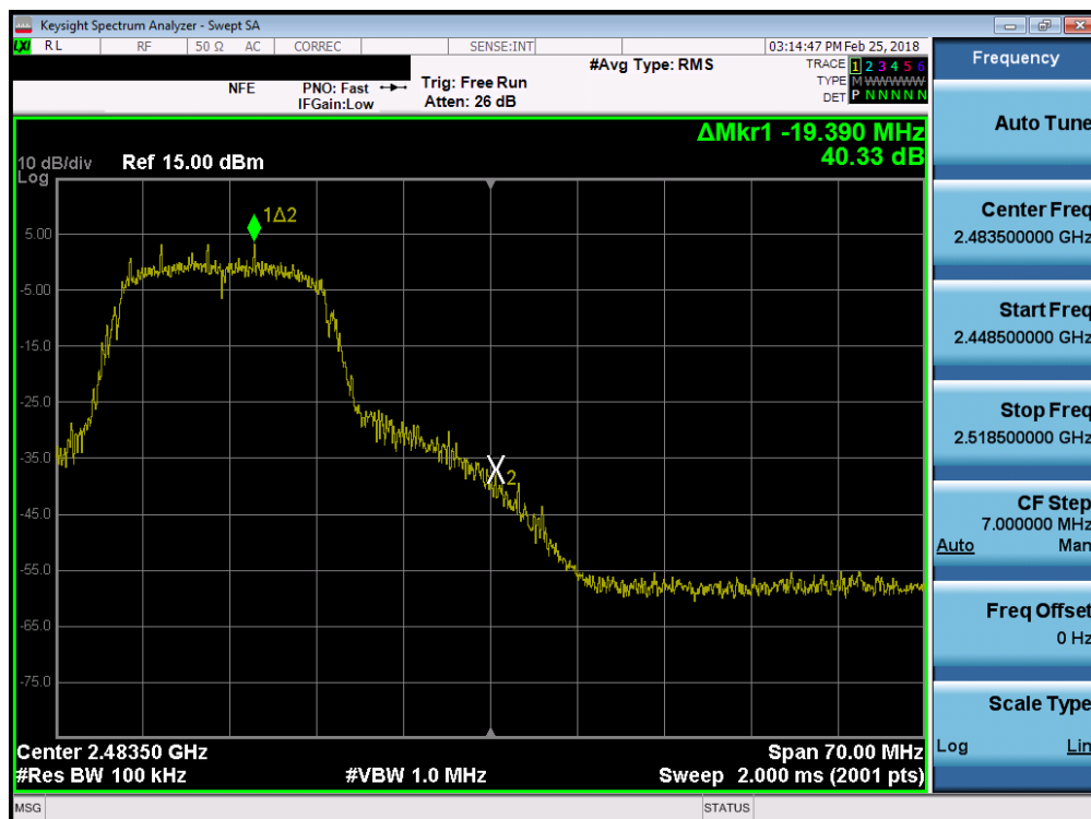
Plot 7-22. Band Edge Plot (802.11g – Ch. 11)
