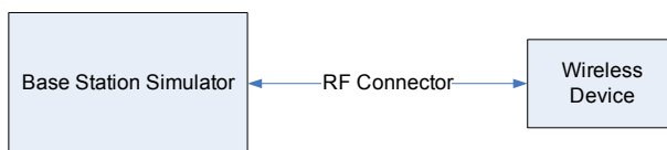
Figure 9-1 Power Measurement Setup
