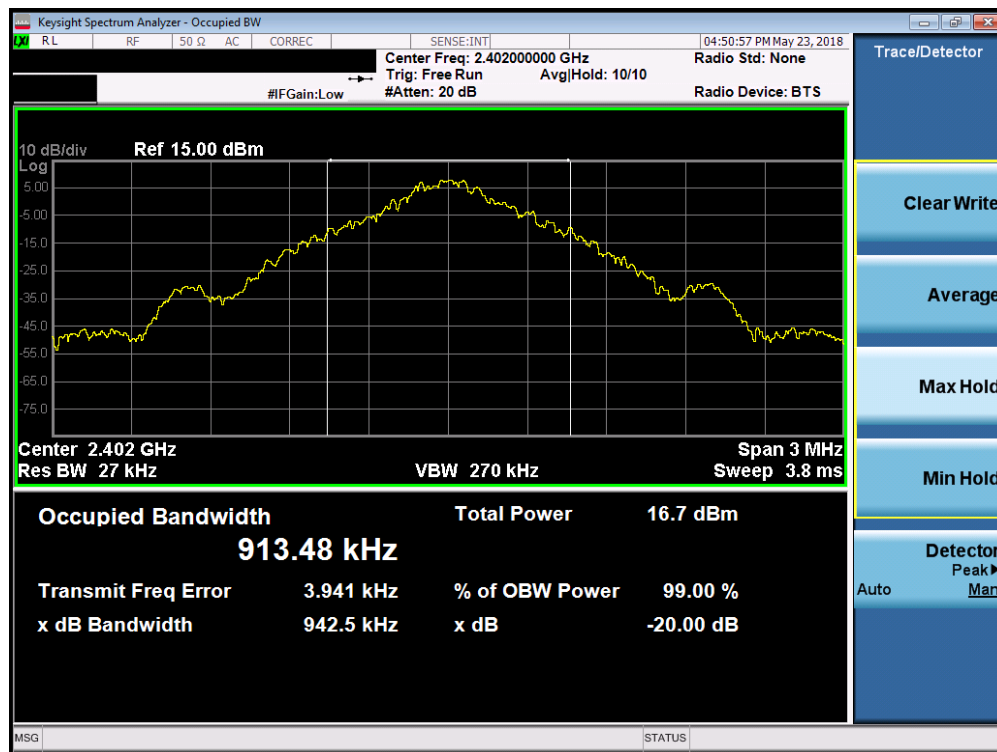
Plot 7-1. 20dB Bandwidth Plot (Bluetooth, 1Mbps – Ch. 0)
