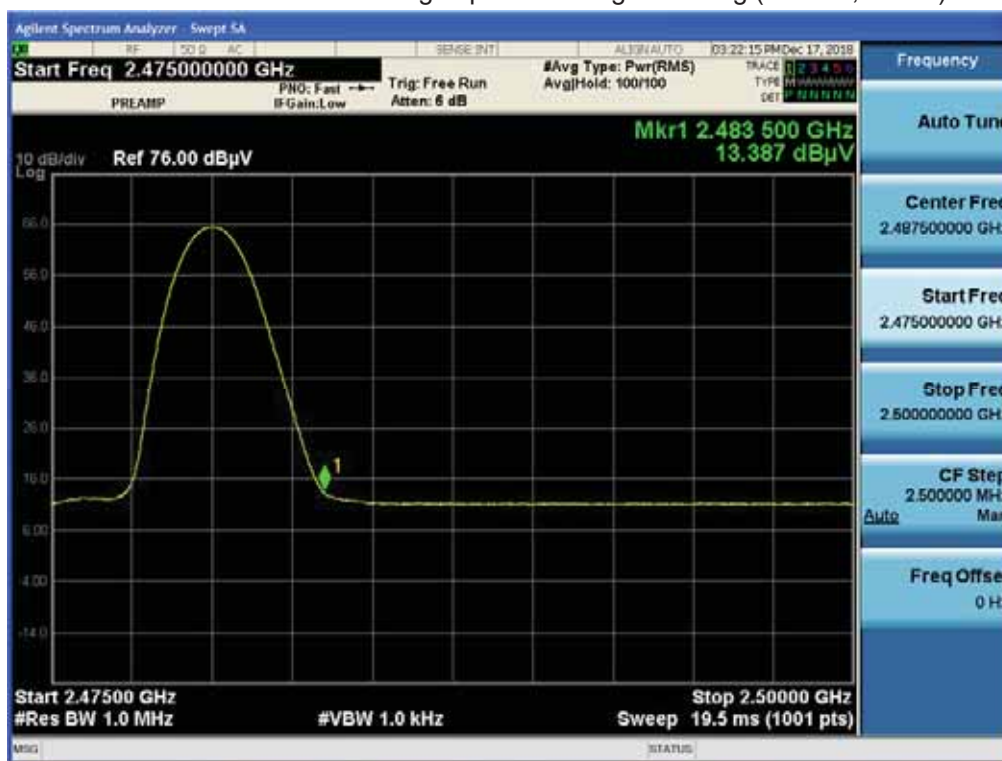
Radiated Restricted Band Edges plot – Average Reading (8DPSK, Ch.78)
