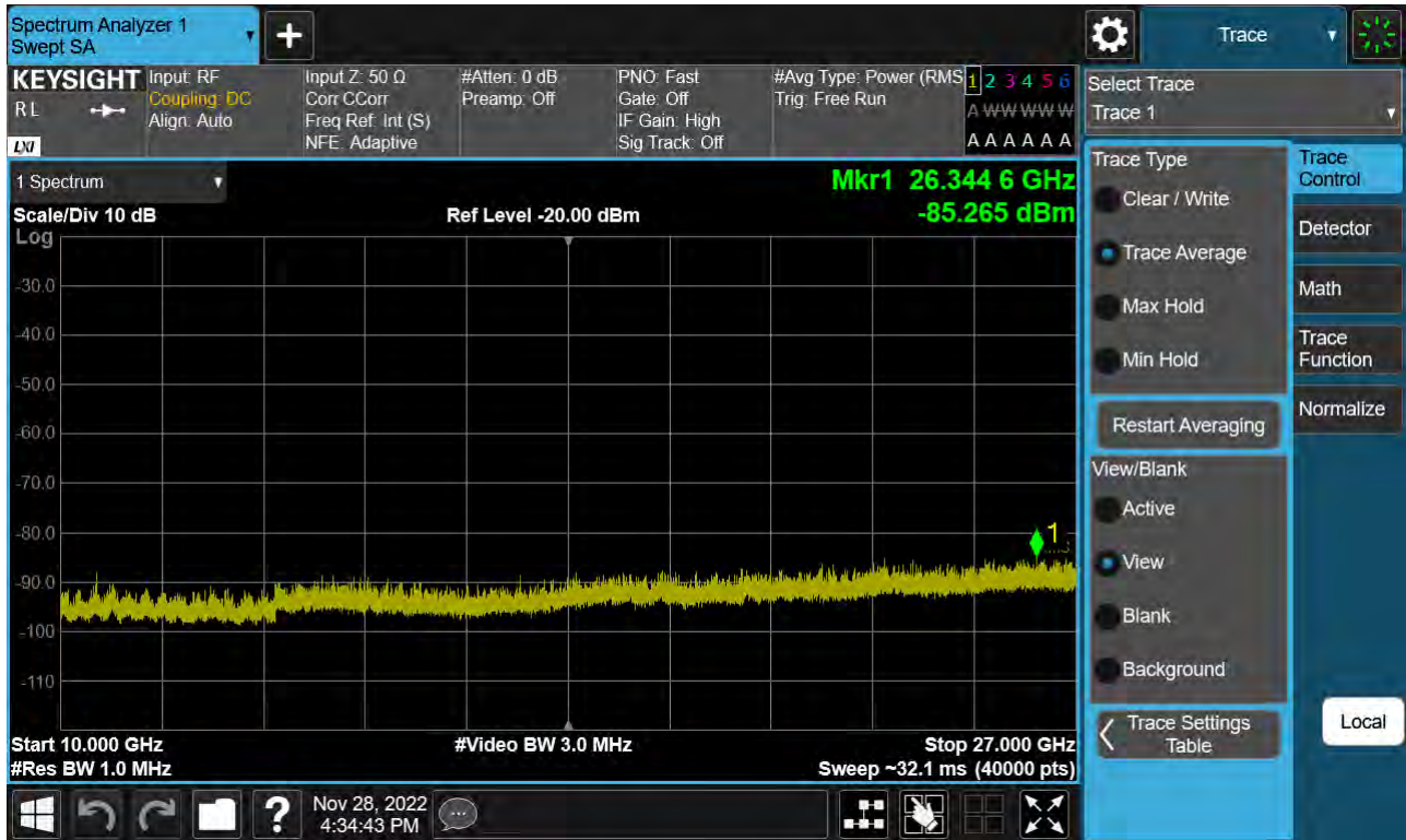
Sub6 n41. Conducted Spurious Plot 2 (50 MHz Ch.504204 BPSK RB 1)
