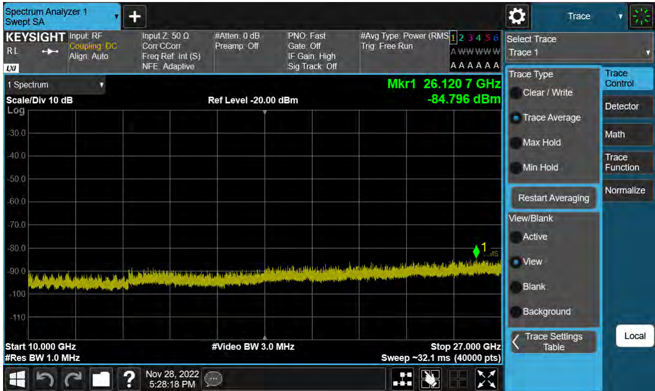
Sub6 n41. Conducted Spurious Plot 2 (90 MHz Ch.508200 BPSK RB 1)
