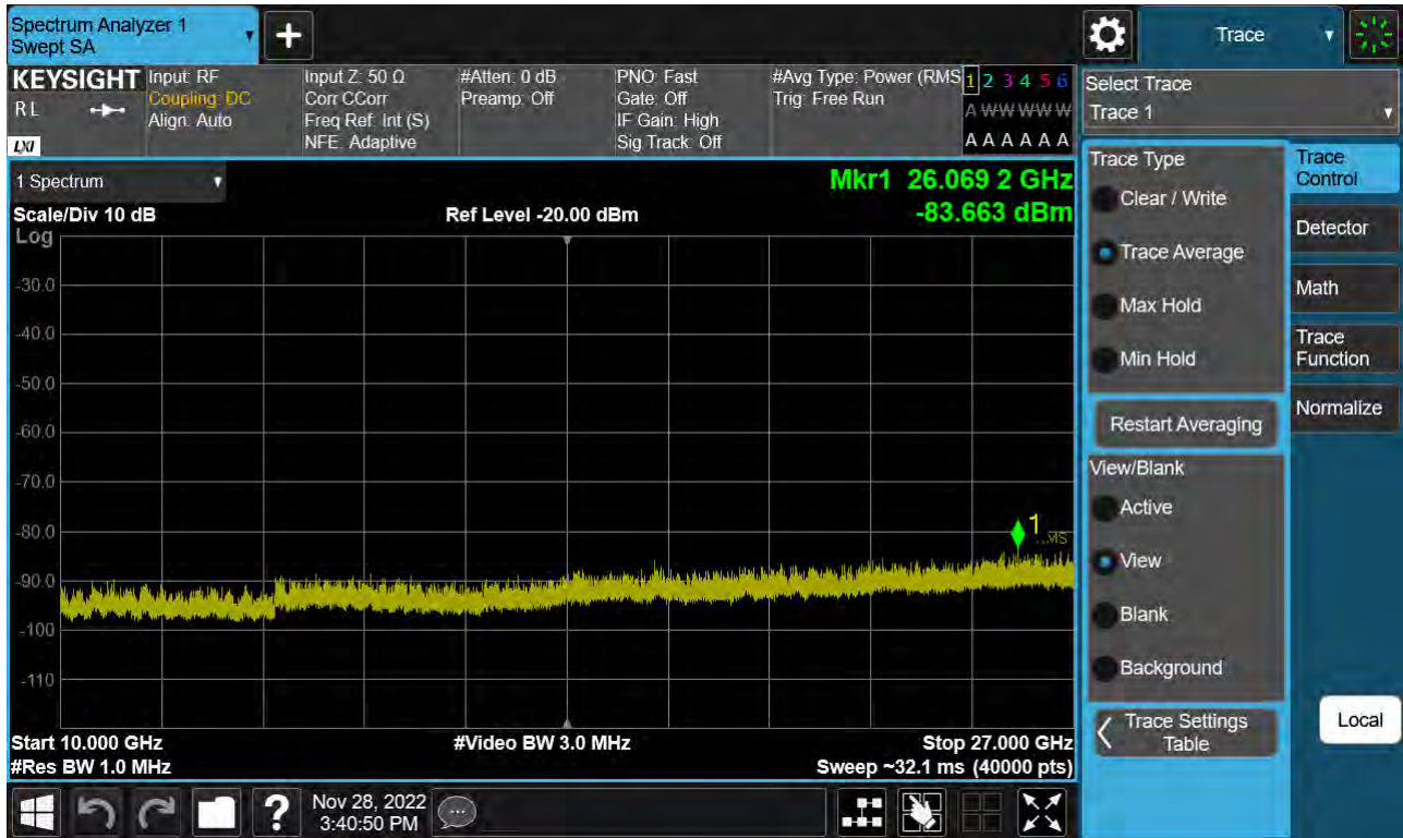
Sub6 n41. Conducted Spurious Plot 2 (15 MHz Ch.500700 BPSK RB 1)
