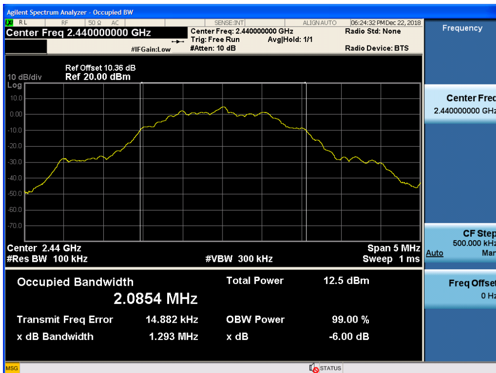
6 dB Bandwidth plot (Mid-CH 19)
