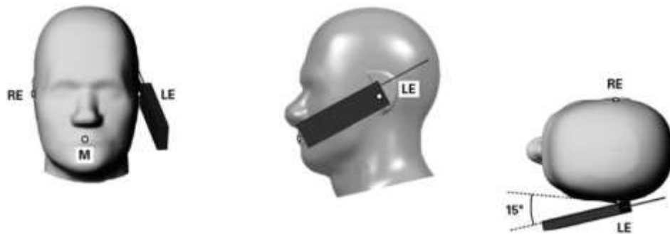
Figure 8.5. Tilt 15° position of the wireless device
