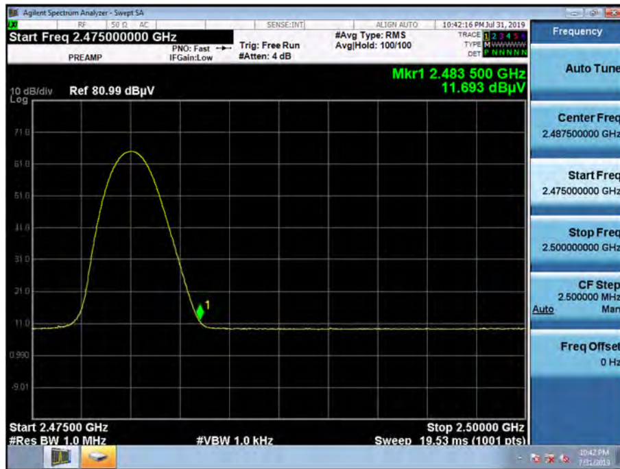
Radiated Restricted Band Edges plot – Peak Reading ( \pi/4 DQPSK, Ch.78)
