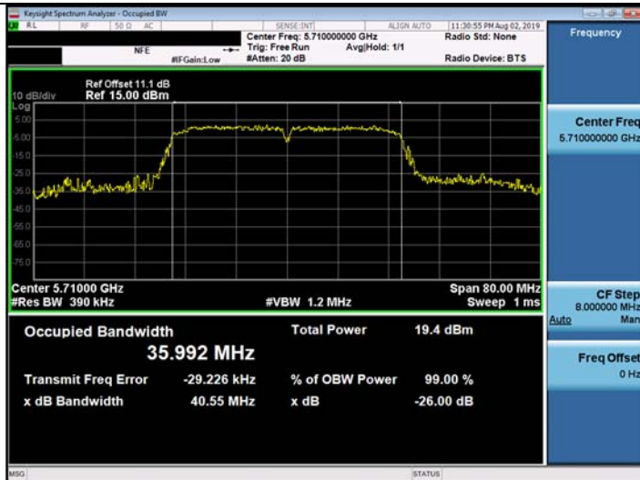
802.11n_HT40 UNII 2C BAND 26dB Bandwidth(CH 142)
