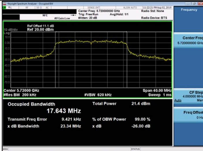
802.11ac_VHT20 UNII 2C BAND 26dB Bandwidth(CH 144)
