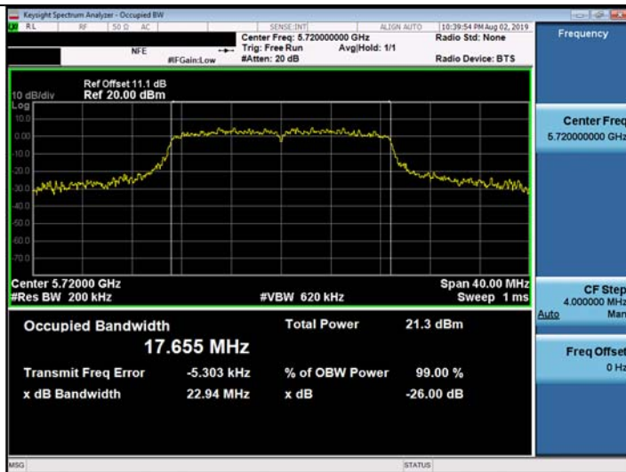
802.11n_HT20 UNII 2C BAND 26dB Bandwidth(CH 144)
