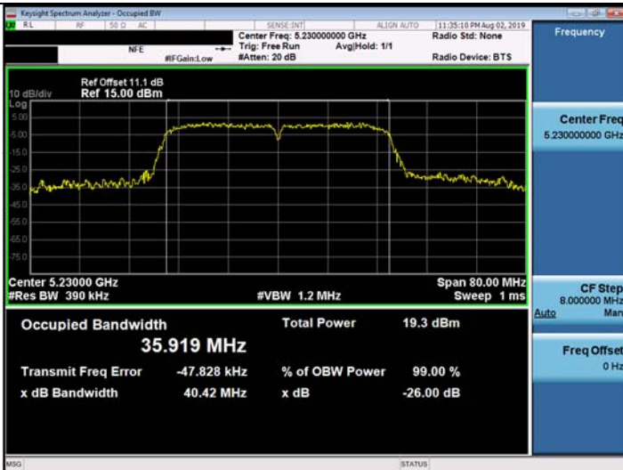
802.11ac_VHT40 UNII 2C BAND 26dB Bandwidth(CH 142)
