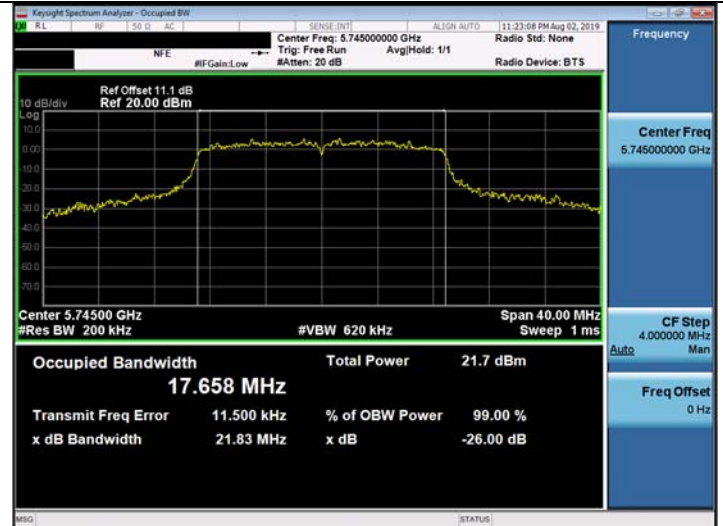
802.11ac_VHT20 UNII 3 BAND 26dB Bandwidth(CH 149)
