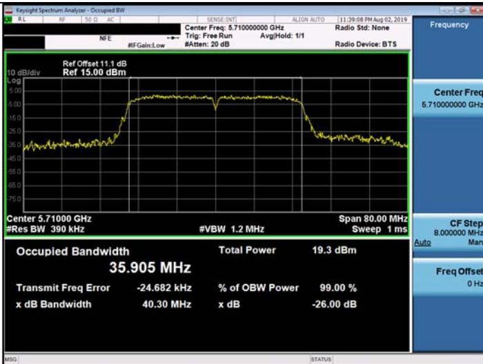
802.11ac_VHT40 UNII 2C BAND 26dB Bandwidth(CH 142)
