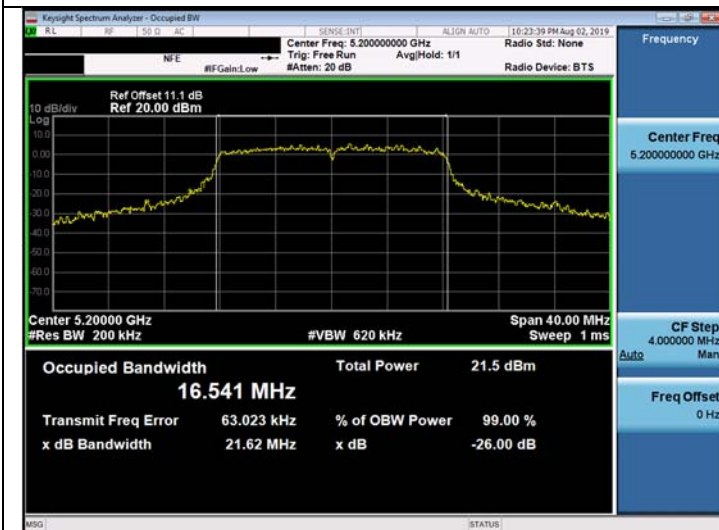
802.11a UNII 2C BAND 26dB Bandwidth (CH120)
