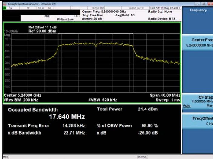
802.11ac_VHT20 UNII 2C BAND 26dB Bandwidth(CH 144)
