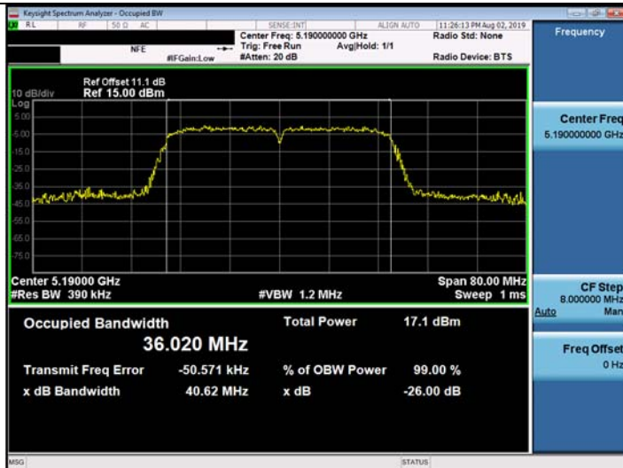
802.11n_HT40 UNII 2C BAND 26dB Bandwidth(CH 142)
