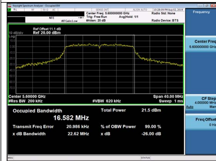
802.11a UNII 2C BAND 26dB Bandwidth (CH120)
