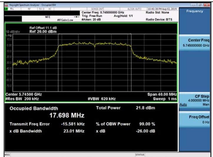
802.11n_HT20 UNII 3 BAND 26dB Bandwidth(CH 149)
