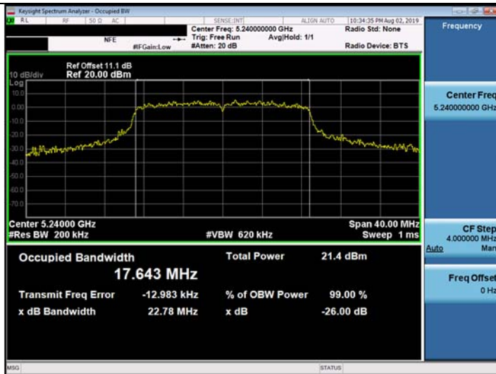
802.11n_HT20 UNII 2C BAND 26dB Bandwidth(CH 144)
