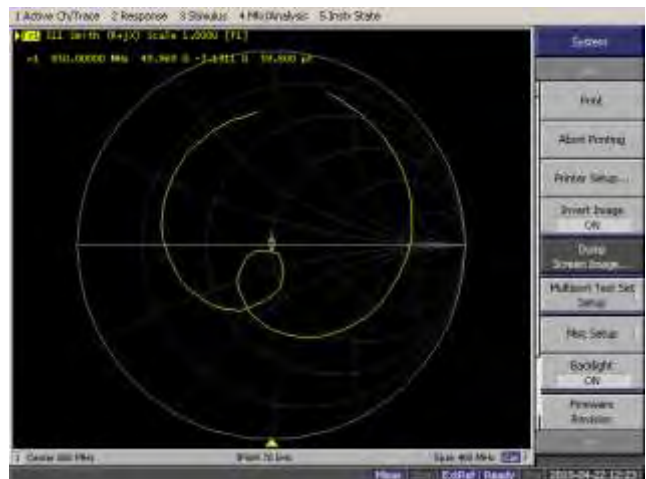
< Figure 2. Measurement result of Head Impedance>
