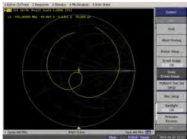
< Figure 2. Measurement result of Head Impedance>
