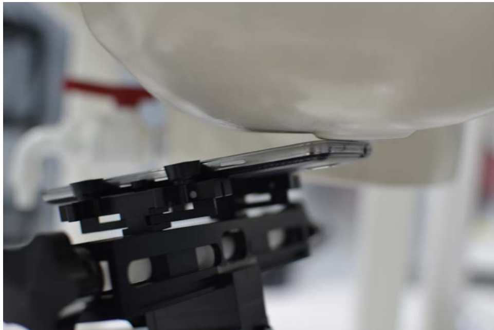
SAR Test Setup Photo 4 – Left Tilt
