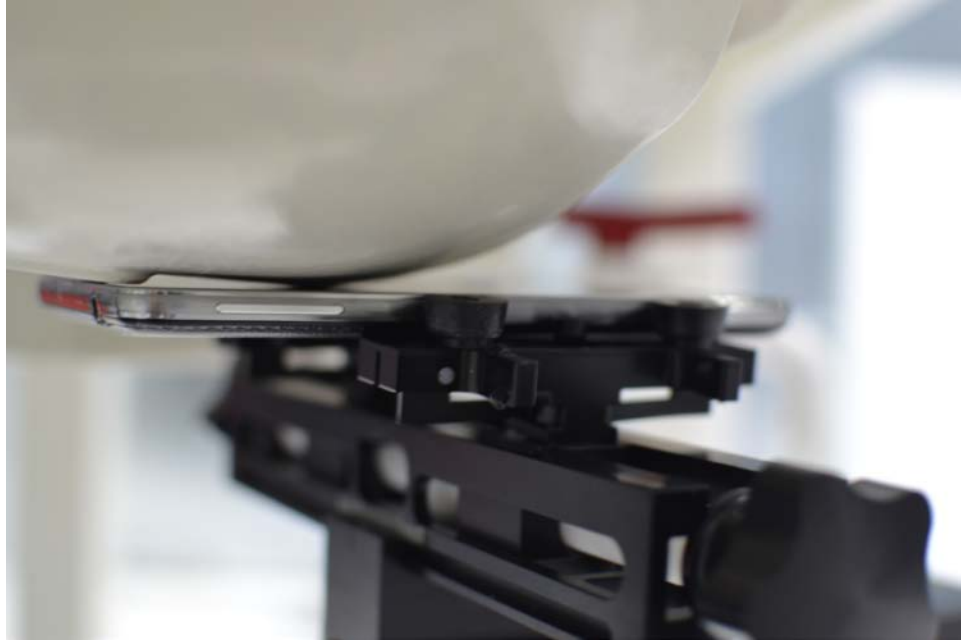
SAR Test Setup Photo 1 – Right Cheek
