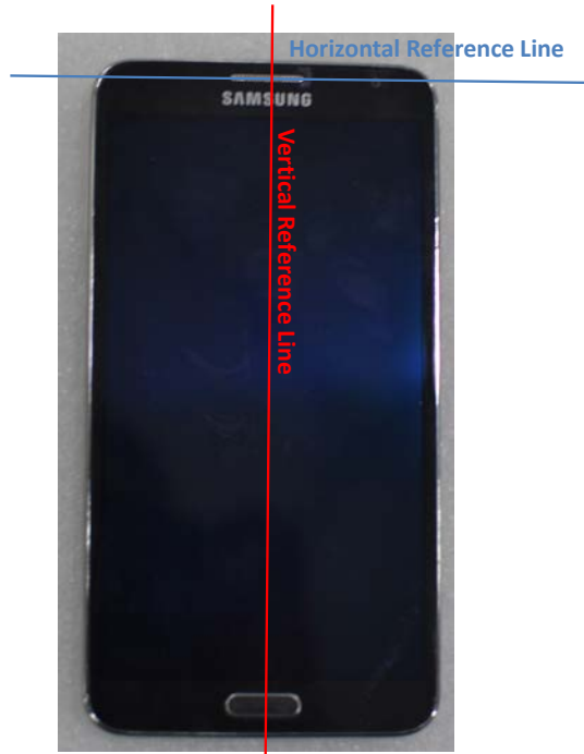
SAR Test Setup Photo 11 – DUT Reference lines
