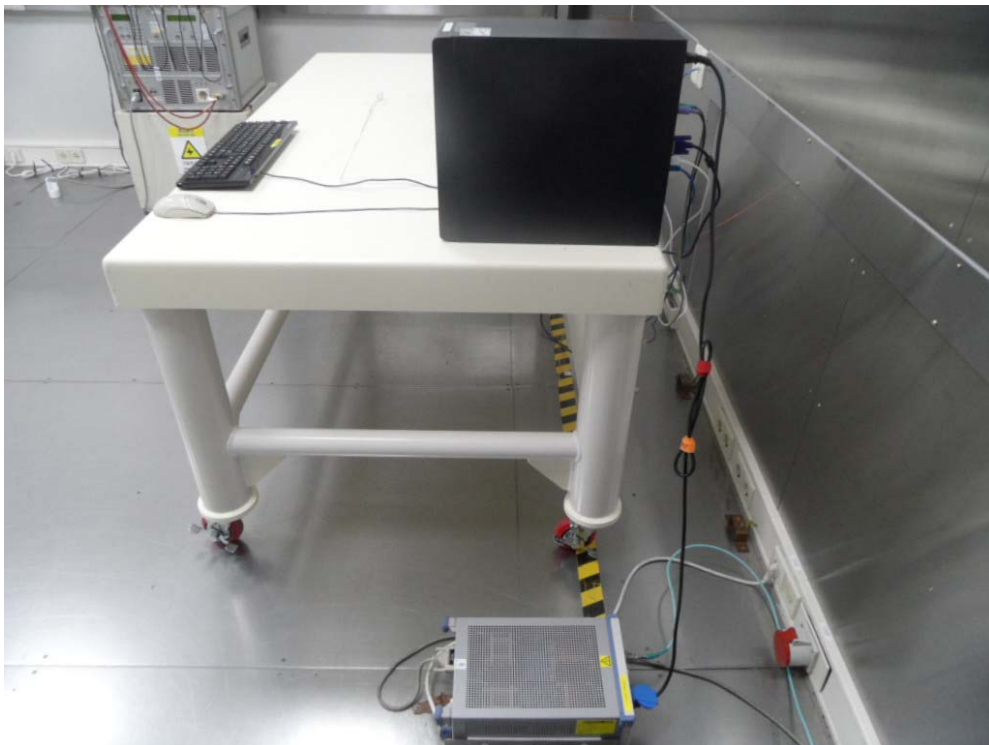
[ Conducted Disturbance – Rear ]
