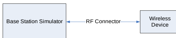
Figure 9-2 Power Measurement Setup
