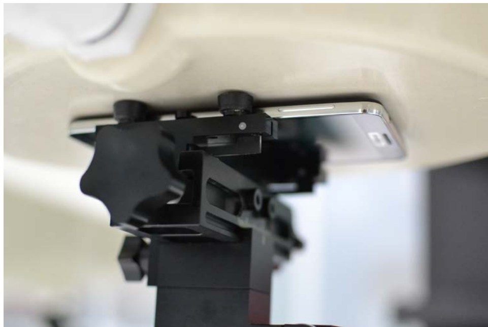
SAR Test Setup Photo 6: Back at 0 mm
