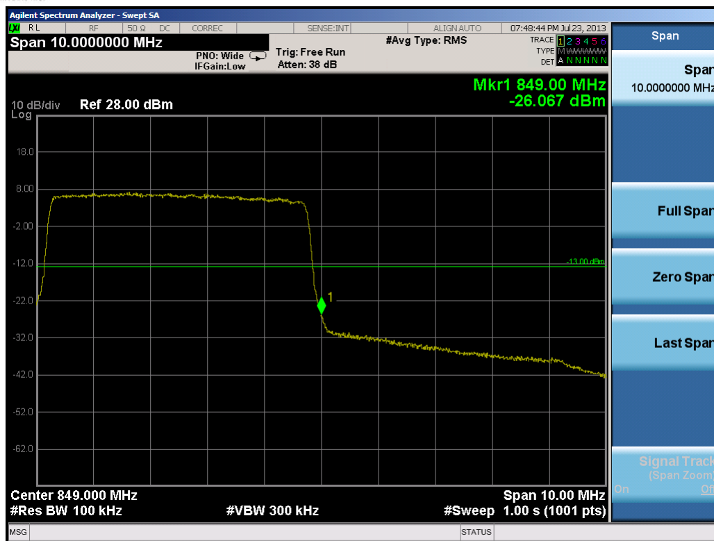
Plot 8-10. Upper Band Edge Plot (5.0MHz QPSK – RB Size 25)
