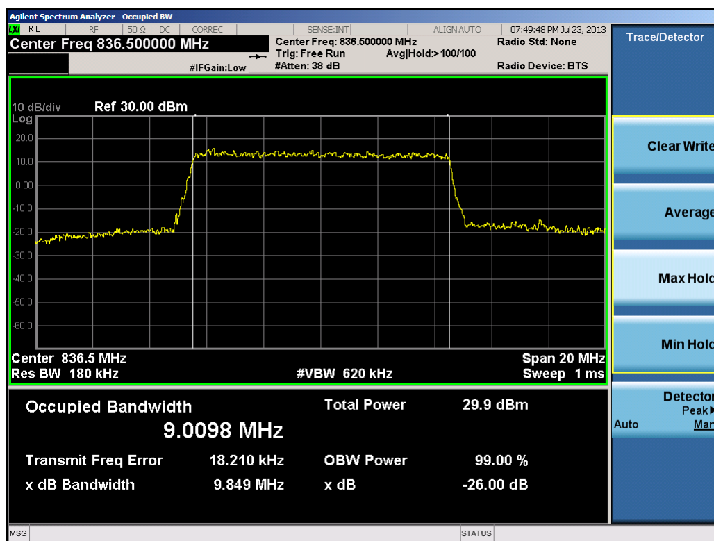
Plot 8-13. Occupied Bandwidth Plot (10.0MHz 16-QAM – RB Size 50)
