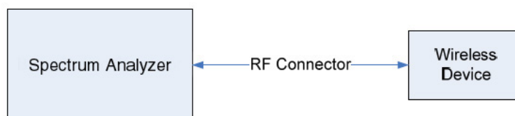
Figure 6-1. Test Instrument & Measurement Setup
